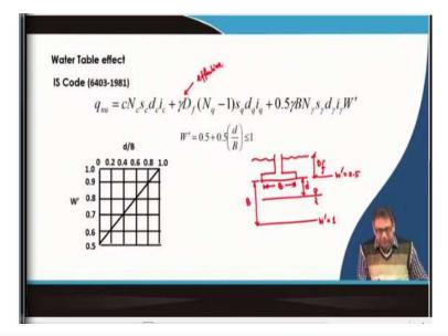
So, now as I mentioned we have to linearly interpolate the value if the water table is from the base to a depth of B, then we have to linearly interpolate from 1 to 0.5. So, or we can use this chart also, so suppose if what is the d, so this is your foundation, this is the base, this is the depth of foundation and say suppose this is the distance B, width of the foundation is B.
