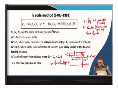
Bearing capacity equation by which we can determine the net ultimate bearing capacity. So, this is the equation which is similar to the general equation that we have discussed. Here also  $s_c$ ,  $d_c$ ,  $i_c$  that means the shape factor, depth factor, inclination factor those are proposed. And the  $N_c$ ,  $N_q$ ,  $N_\gamma$  values are similar to the values proposed by Vesic, we have to use.
