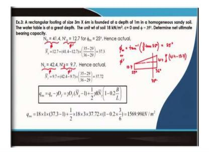
Now if the  $\phi$  of the soil is greater than 36°, then it will be a general shear failure and if  $\phi$  of the soil is less than 29° then there will be the local shear failure. Now if the  $\phi$  of soil is within 29° and 36°, then how we can calculate that. So, in such case this is the example in such case we can determine the bearing capacity by using both the theories.
