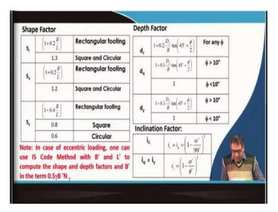
For the shape factor, depth factor, inclination factor you will use these charts. The shape factor you will use for rectangular footing, square and circular footing, rectangular for square footing  $s_q$  and  $s_{\gamma}$  also you will get from this table. Depth factor also I will get from this table for any  $\phi$ , if  $\phi \ge 10^{\circ}$  for this equation.
