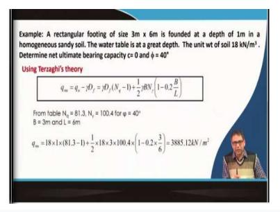
So, now this is the first example problem where a rectangle footing of size 3 m × 6 m is placed at a depth of 1 m in a homogeneous sandy soil, the water table effect is not considered. Because water table is at a great depth, I mean below depth of *B*, the unit weight of soil is 18 kN/m<sup>3</sup>. Determine the net ultimate bearing capacity when c = 0,  $\phi = 40^{\circ}$ .
