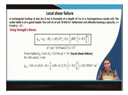
So, in the previous example problems the general shear failures are considered ok. So, now if the soil is in a local shear failure then what will happen? That means here  $\phi$  is 22° which is less than 29°, so it will be a local shear failure. Then what will happen, how we can calculate the bearing capacity? So, I have discussed as per Terzaghi's bearing capacity theory we have to take the  $\frac{2}{3}c$  but here *c* value is 0.
