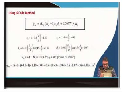
Then as per IS code here water table effect is not considered, so W' is taken as 1. So, this is the bearing capacity factor which is same as Vesic and then the shape factor and depth factor is taken from the table and then I will get this value.
