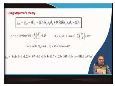
So, using Meyerhof's equation this is the equation I will get the net ultimate bearing capacity. So, I will use these shape factors and depth factors because I will get these things from the table that I have given for Meyerhof's bearing capacity equation. I will get the  $N_q$  and  $N_\gamma$  value corresponding to  $\phi = 0^\circ$ . For general shear failure and I will get this value, for net ultimate bearing capacity as per the Meyerhof's bearing capacity theory.
