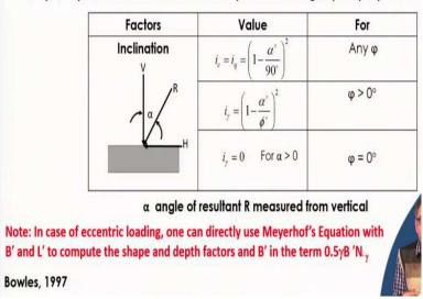
Shape, depth, inclination factor for the Meyerhof's bearing capacity equation:
