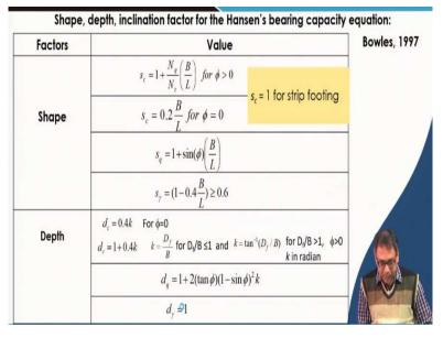
So, now here we can determine the shape factor, depth factor and inclination factor as per Hansen's bearing capacity equation. So, shape factor you can get by this equation. Now if  $s_c = 0.2 \frac{B}{L}$  for  $\phi = 0^\circ$ , for  $\phi > 0^\circ$  we will use this equation okay. Similarly, we can calculate  $s_q$  and  $s_{\gamma}$ , remember that this  $s_{\gamma} \ge 0.6$ . So, if  $s_{\gamma}$  is coming say less than 0.6, then we have to use 0.6, remember that.
