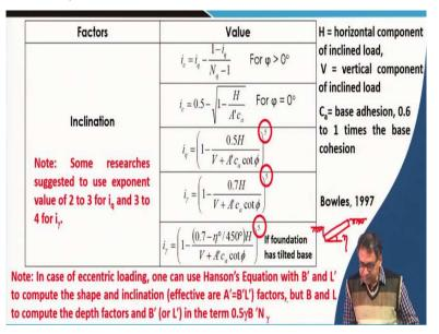
Now, this is the inclination factor, we will calculate the inclination factor. So inclination factor  $i_c$ ,  $i_q$  we will get by using this equation,  $i_q$ ,  $N_q$  I will get from the chart because  $N_q$  is similar to the Meyerhof's  $N_q$ . So from that chart we can get the  $N_q$  value and similarly here also  $N_c$  and  $N_q$  also we will get from the chart because  $N_c$  and  $N_q$  both the same as suggested by Meyerhof.
