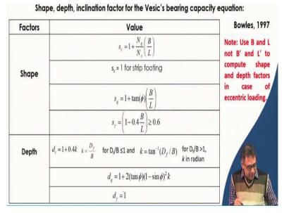
And this is the table which is similar to Hansen's theory, but remember that in case of Hansen's if  $\phi = 0$  our particular equation is given, but here it is not given. So that means if you use Hansen's equation for  $\phi = 0$ , then the table that is given, so you have to use that table, then you have to use that equation which is given for  $\phi = 0$ , but here in Hansen and Vesic you can see that type of equation is not given for  $\phi = 0$ .
