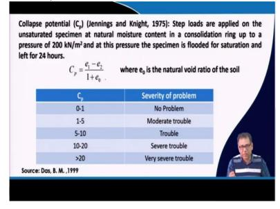
Now that there is a term called collapse potential, so by which we can identify that if the soil has some problem related to this collapse. So, this collapse potential is what? That we apply step loads on the unsaturated specimen at natural moisture content in a consolidation ring up to a pressure of 200 kPa. So that means, we place the soil sample in a consolidation apparatus, or Oedometer and in the consolidation ring under the natural moisture content condition or under unsaturated condition.
