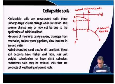
So, now, what is the collapsible soil? The collapsible soils are the unsaturated soil that undergo large volume change when they are saturated. Now, this volume change may be or may not be due to the application of additional load. So that means, suppose soil is unsaturated condition and then when we saturate that soil suddenly there is a huge volume change, large volume change even if we have not applied the additional load on the soil.
