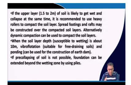
And then if the upper 1. 5 m to 2 m of the soil layer is likely to get wet and collapse at the same time, then it is recommended to use the heavy roller to compact the soil layer. Suppose if the collapsible soil layer is a shallow depth or shallow, the thickness is small then we can apply the heavy roller to compact this soil. Suppose, as I mentioned, so this soil has very high void ratio.
