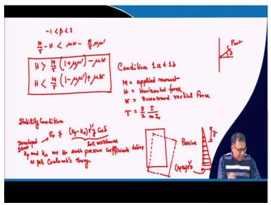
So that condition is this one that your *H* should be greater than  $\frac{M}{r}(1 + \mu\mu') - \mu W$  or *H* should be less than  $\frac{M}{r}(1 - \mu\mu') + \mu W$ . Now these are the values and I have discussed what are these values. Now the next condition for the stability condition.
