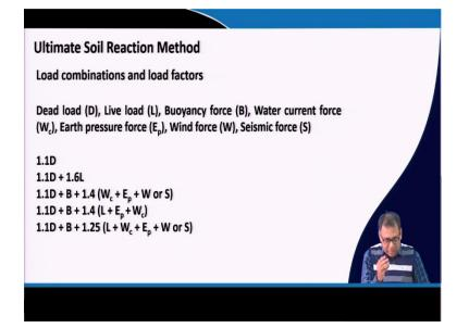
So, next method that I will discuss is the ultimate soil reaction method. So, ultimate soil reaction method is another method by which also you can determine or we can check the stability of the well. So, in this method, the load combinations and the load factors which are recommended are as follows. So, what are those load factors, so here the different loads will act on the well.
