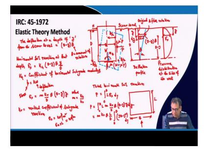
For example, that conditions so you can see that this well is rotating from left to right side or you can say it is rotating in clockwise direction. So that means that both side there are soil. So, one side will be passive another side will be active similar to that I have discussed during Terzaghi's analysis. So, here the right side will be the passive condition and left side will be the active condition. So, if I draw that condition suppose this is the original position of the well.
