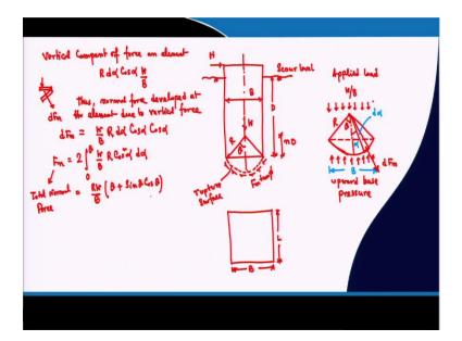
So, next one is that for this particular method that will consider that this is the well. So, this is well this is the scour level here the H is acting in this direction this is the center line, this is B and this one is the depth well below the scour level. And here this method assumes that this well will rotate with the point and say this point is this one, and that point is at a height of nD from the base of the well.
