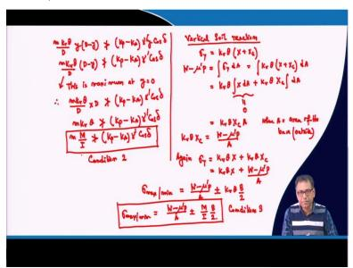
So, if I write that  $\sigma_x$  value, so this will be  $m \frac{K_v}{D} \theta (D - y) y$  that should not be greater than  $(K_P - K_A) \gamma' y \cos \delta$ . So, further we can write  $m \frac{K_v}{D} \theta$ , so y y will be cancel out and D - y should
