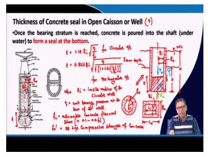
Now, today I will discuss that how we can determine the thickness of the concrete seal in open caisson or well. So, as in my previous lecture, I have already discussed that when the bearing strata is reached for open caisson when the concrete is poured inside the shaft under water to seal at the bottom, so that means, here you can see. So, this is the shaft and these are the places where the concreting is done to seal the bottom and then once the concrete hardens.
