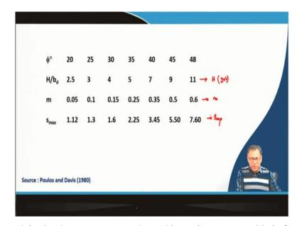
So, now, let me explain that how we can use these things. So, suppose this is for the  $\phi$ . So, this is H for different  $\phi$ , this is the  $\frac{H}{b_d}$ . So, we know the  $b_d$  we talked about the diameter of pile base, then using these table different  $\phi$  value we will get the H. So, from here, we will get the H value, from here because we know that  $d_b$  and we will get the H value and we will get the m value also here and we will get the  $s_{\text{max}}$  also here.
