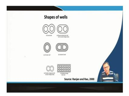
And then what are the different shapes of the well. So, circular shape is the most common shape of the well in addition to that there is rectangular shape of the well and other shapes are also described here. So, these are the different shapes of well.
