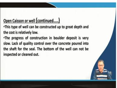
Now this inside portion is filled with sand. Now, this type of well can be constructed up to a great depth, any depth and its cost is relatively low. The progress of construction in boulder deposit is very slow. So, the advantage is that it can be installed up to any depth but cost is very low. But the disadvantages are the progress of construction in boulder deposit is very slow, the lack of quality control over the concreting, because now concreting is done underwater.
