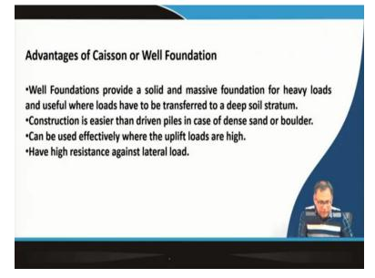
So, next one I will discuss the well foundation. So, this well foundation is sometimes called as the caisson foundation also. So, the advantage of these caisson or well foundation, this well foundation provide a solid and massive foundation for heavy loads and useful where loads have to be transferred to a deeper soil strata. The construction is easier than the driven pile in case of dense sand and the boulder.
