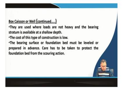
So, these are used where loads are not heavy and bearing strata is available at a shallow depth, the advantage is the cost of this type of construction is low and the disadvantages are the bearing surface or foundation base must be level or should be levelled before it is installed then care has to be taken to protect the foundation bed from the scouring action.
