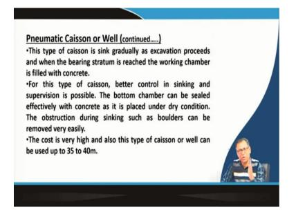
So, now this type of caisson is sunk gradually as excavation proceeds and when the bearing strata is reached the working chamber is filled with concrete. So that is acting as a bottom plug. So that working chamber is sealed. Now for this type of caisson, better control in sinking and the supervision is possible. Now bottom chamber can be sealed effectively because now there is no water when the concrete is in done for the seal of the bottom plugs because it is done under dry conditions.
