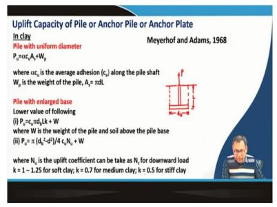
Or I can give you the anchor pile or anchor plate because uplift capacity of the pile I have discussed in the last class. And then you can determine but there is another approach also where you can determine the uplift capacity of the pile or you can say it is the anchor pile or uplift capacity of anchor plate or uplift capacity of foundation also. So, that is given by Meyerhof and Adams in 1968 which is for clay and it is same as the uplift capacity of the pile.
