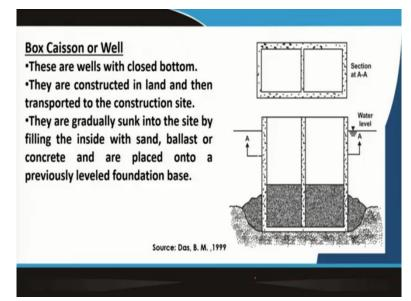
So, the next one is the box caisson where the bottom portion is closed, but top portion is still open. And they are constructed in the land and then transported to the construction site, the previous one was constructed in the site itself, but here it is constructed in the land and then transported to the construction site. And they are generally sunk into the site by filling inside the sand, ballast or concrete because now the bottom is sealed.
