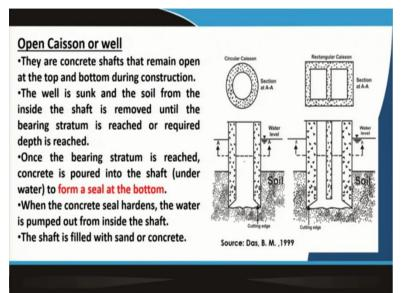
So, now this well foundation can be different types. So, first one is the open well or the open caisson. So, here you can see this is the plan and the cross section. So, this is a circular caisson and this is a rectangular caisson. And here this is a section. So, this is the soil where the foundation we have to install and definitely above that it is the water table or water, generally these type of foundation are suitable for the beach structure.
