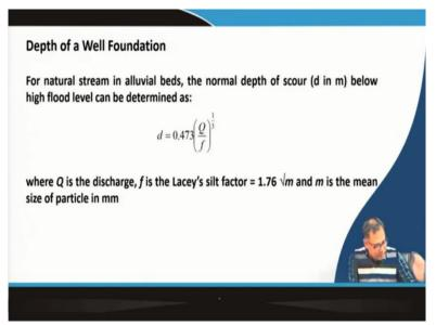
So, now, we are talking about how we can determine the depth of a well? How we will decide that, so to know that we have to determine what would be the scour depth for a particular site, so that scour depth we can determine by Lacey's formula, so *d* is the scour depth. So, *Q* is the discharge and *f* is the Lacey's silt factor, which is generally  $1.76\sqrt{m}$ , *m* is the mean size of the particles in mm, *Q* is the discharge. So, now, by using this equation you will get the scour depth
