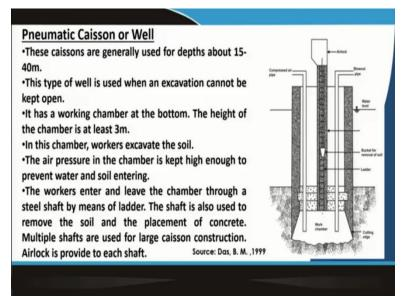
The next one is the pneumatic caisson or the well. So, these types of caisson are generally used for up to a depth of 15 m to 40 m. So, this type of well is used when the excavation cannot be kept open because what is the difference between these one and the first one, in the first one both bottom and top are open. So, sometimes it is not possible that the excavation cannot be open because soil
