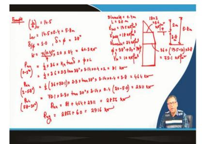
Now, let me solve one particular example problem. So, this example problem will help you to determine or to know the uplift capacity of the pile. So, for the diameter of the pile was given 0.4 m and variation is this is the water table, this is the critical and this is the uniform. So, these are the three variations here the water table is present here which is at a depth of 2 m diameter is 0.4 m then the length of the pile is 20 m.
