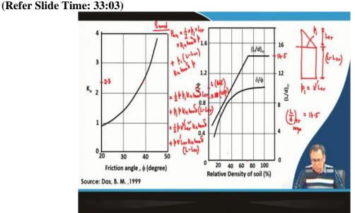
Now, this is for the cohesive soil now, for the granular soil, how we can calculate this value and also that means, for the granular soil there will be again the critical depth we have to calculate. So, this is the critical depth where this is the critical length,  $L_{cr}$ , this is  $L - L_{cr}$ . So, this is for the granular soil or sand the initial was for the clay and this is for the sand. Now, how I will calculate the critical length?
