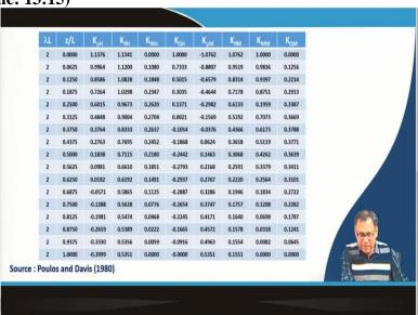
Which is similar to the equation for finite beam. So, but here that  $K_{\theta H} = 0$   $K_{\theta M}$  at z = 0 that is also close to  $K_{\theta H}$  so, which is not 0 actually  $K_{\theta H}$  is not 0 at z = 0 this is z = 0 so, that is that is why you have to calculate or you have to put these values depending upon what is your  $\lambda L$ .
