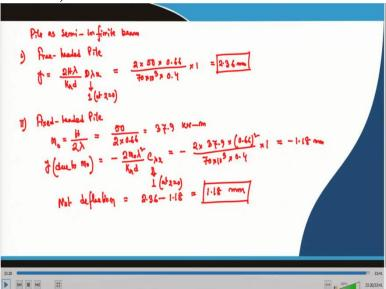
Now, if the next pile is as semi-infinite beam: The pile as semi-infinite beam so, you use the same problem, but here again for free-headed pile the equation of  $y = \frac{2H\lambda}{k_h d} \times D_{\lambda z}$  so,  $D_{\lambda z} = 1$  at z = 0 but for any other z, I have discussed that how to calculate this coefficient for any depth or any distance. So, you have to convert this in radiant.
