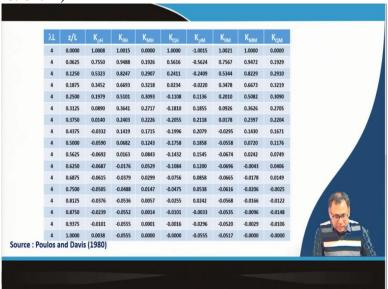
So, we will go for the pile and as I have already discussed that how we will get this  $K_{\rho H}$  to the  $K_{QM}$  coefficient values with respect to different  $\lambda L$  and z/L, z is any depth and L is the length of the pile and  $\lambda$  I have already discussed. So, this is  $\lambda L = 2$ , this is  $\lambda L = 3$ , this is for  $\lambda L = 4$ , this is for  $\lambda L = 5$ .
