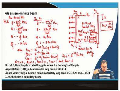
Now, we will go for the pile as a semi-infinite beam. So, when the pile is called the long pile, so, if the  $\lambda L > 2.5$ , then the pile can be called as a long pile where L is the length of the pile. So as per Hetenyi a beam is called the long beam if  $\lambda L > 3.14$  as per Vesic the beam is called moderately long beam if  $\lambda L > 2.25$  and  $\lambda L < 5$  and if the  $\lambda L > 5$  then the beam is called long beam.
