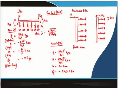
And before we go to the semi-infinite beam part so, there is a small correction and this that correction in expression for slope due to moment will be  $\lambda^3$ . So, this is  $\lambda^3$ . So, that this is the correction.
