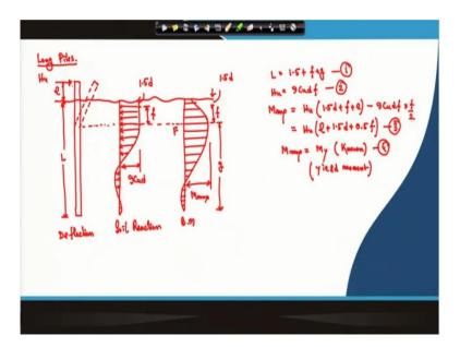
So, for the long pile what will happen? This is for the long pile; previous one is for the short pile. And for the long pile same if I take the ground surface, this is the ground surface and we have a pile which is a long pile. Here also  $H_u$  is acting at a height of e and here again this is the *L* length of the pile. So, here the total pile will not rotate because as the pile is long. So, lower part of the pile will be very rigid, it will not move like the short pile.
