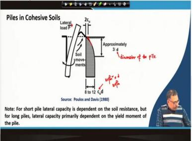
So, I will discuss the ultimate lateral load carrying capacity of piles in two types of soil first one is the cohesive soil and then the second one is for cohesionless soil. And I will also discuss the lateral load capacity of the pile for two types of piles one is the short pile, one is the long pile. So, in general that if pile is subjected to lateral load in cohesive soil then we will get this type of distribution. So, what is that distribution?
