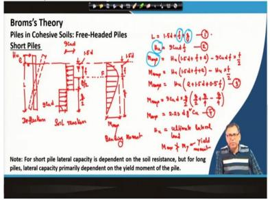
So, based on that, Broms proposed different soil pressure distributions for short piles and the long piles, pile in cohesive soil and the cohesionless soil. So, I will discuss first Broms's theory. So, Broms has suggested different pile soil pressure distribution for different types of piles that means, it can be short pile, long pile, it can be free headed, it can be fix headed. So, first I will discuss about the piles in cohesive soil which is a free headed pile and a short pile.
