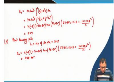
So, I have determined that 13.81 m is the  $L_1$  value, so  $F_n$  I can calculate the expression is given if I integrate so I will get that expression that is  $pK \tan \delta \int_0^{L_1} (\bar{q}_0 + \gamma' z) dz$ . So, now if I put the limit so, this will be  $pK \tan \delta (\bar{q}_0 L_1 + \frac{1}{2}\gamma' L_1^2)$ . So, now we will put this value p is the perimeter which is  $\pi d$ .
