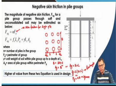
So, this is the group pile. So, the negative skin friction cases are same as I have discussed for the single pile. So, only difference that how we can determine the negative skin friction for the group pile the same way we can determine the negative skin friction for the group pile as we did it for the group pile load carrying capacity. So, first we calculate the negative skin infection for the single pile then you have to multiply it with the number of piles.
