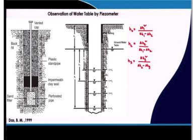
So, this is the expression by which we can determine the water table position of clay soil by using piezometer.
