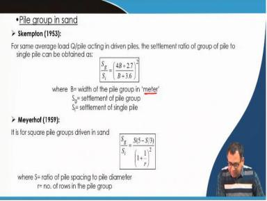
So, now pile group settlement also we can determine based on the single pile load test data suppose if I know the single pile settlement, then based on these equations we can determine the pile group settlement also. So, this is the settlement of the pile group, we can determine the settlement of single pile,  $S_i$  and B is the width of the pile group and this is the equation remember that we have to express B in meter.
