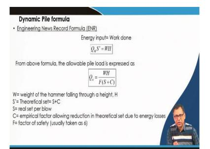
So, then we can use the dynamic pile formula by which also we can determine the load carrying capacity of the pile. So, there are several equations which are given. So, I am discussing two of them. So, the one is the engineering news record formula or ENR formula. And basically, here we are applying the hammer blow because it is done on driven piles and we have applied the hammer blow and then we apply the energy. And so that means the work done we have to equate with the input energy.
