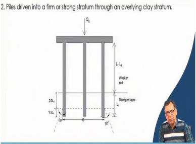
Now if the pile is resting in a stronger layer and the top layer is a weak layer then the raft we have to place at a depth of  $\frac{2}{3}L_1$  from the top of the stronger layer and  $L_1$  is the thickness of the stronger layer. So, suppose this is a weaker layer and this is a stronger layer, if the strength difference is not that much significant, then we will consider it as a homogeneous soil.
