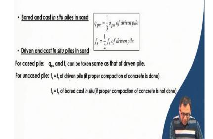
Similarly, for the bored pile because those equations are given for the driven piles. And so for the bored and cast-in-situ piles in sand that  $q_{pu}$  will be  $\frac{1}{3}q_{pu}$  that we have determined by using the already discussed equations for driven pile and friction resistance will be half of the prescribed shaft resistance of the driven pile. But if it is a driven and cast-in-situ pile in sand, then if it is cased, then the  $q_{pu}$  and  $f_s$  are taken same.
