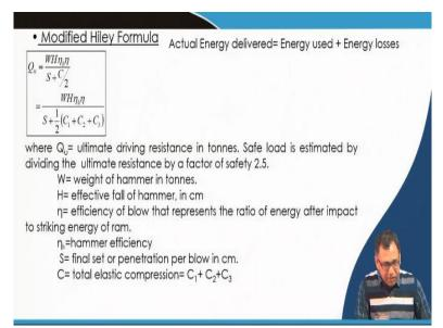
Similarly, there is a modified Hiley formula, where actual energy is equal to energy used and energy loss because previous also equation also energy lost is taken care by this empirical factor C. But here the total delivered is energy used plus the energy loss and based on that determine the ultimate load carrying capacity of the pile. So, again here W and H are the weight of the pile and the height of fall, respectively.
