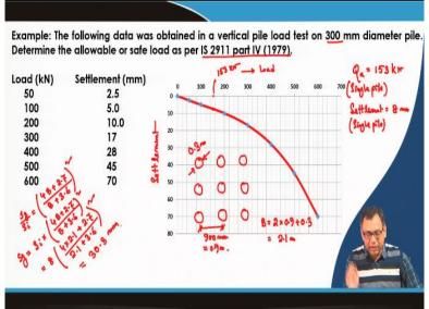
Now, I will solve one example problem, so the same load settlement plots are taken here that used to calculate the load carrying capacity of the single pile. So, that same load settlement curve I used here. So, this is the load settlement curve, so this is the load, and this is the settlement. So, in previous case the same problem, the  $Q_u$  for the single pile was 153 kN and that is the ultimate load carrying capacity of the single pile.
