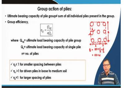
Then now I will go for the group action of the pile. So, suppose we have a pile group of 9 piles, so these ways we can determine the efficiency of the pile. So, first we have to determine the load carrying capacity of the pile group considering the block failure. Block type of failure means that total pile group will fail. So, considering that we will calculate the load carrying capacity of the pile group.
