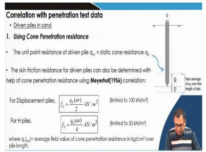
Then we can determine the load carrying capacity of the pile by using the penetration test data that mean by using cone penetration resistance. By cone penetration distance, if we take the average of 1*D* below the pile tip and 3*D* above the pile tip, total 4*D*, *D* is the diameter of the pile and the average cone resistance is  $Q_c$  that will give us the tip resistance of the driven pile in the average of 3D + 1D, 1D below the tip and 3D above the tip.
