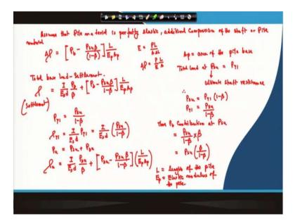
Now, one thing I want to mention that when we are talking about the settlement, now this settlement is the settlement of the pile material + settlement of the soil. If the pile is incompressible then the settlement will be settlement of the soil itself. But if the pile is compressible then the settlement of the pile is due to the settlement of the soil and settlement of the pile material itself.
