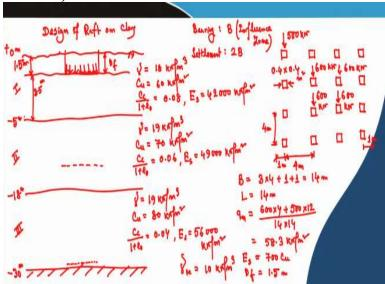
So, this is the soil profile that was taken and for the bearing capacity consideration the influence zone was your 14 m which is *B* and for settlement calculation it will be 28 m. So, that will be just close to the end of the third layer so, up to 29.5 m from the surface. So, now we have taken the weighted average because the variation is not that significant for the  $C_u$  value or the strength parameter.
