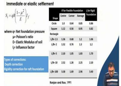
Now, influence factor table is given so, here what I am considering or I am taking that it is a raft foundation, so, it is a rigid foundation. So, directly I can take the,  $I_f$  for the rigid foundation, but as later on I will apply the rigidity correction for consolidation settlement. So, that is why I have decided I will take the centre  $I_f$  for flexible foundation then I will apply the rigidity correction of 0.8.
