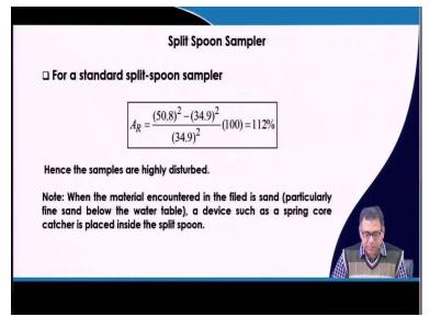
So, the area ratio will be  $\frac{50.8^2 - 34.9^2}{34.9^2} \times 100 = 112\%$ . So, that means the samples that we are collecting by using split spoon sampler are highly disturbed samples.
