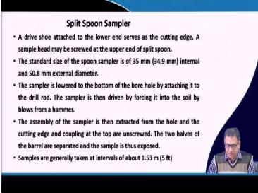
And split spoon samplers. So, this is the description of the split spoon samplers. So, there is a cutting edge in front of the sampler tube and a split spoon sampler with inside diameter of 35 millimeter or 34.3 millimeter, an external diameter is 50.8 millimeter and then the sample is generally taken at an interval of 1.5 meter or 5 foot and these sampler tubes it has 2 halves.
