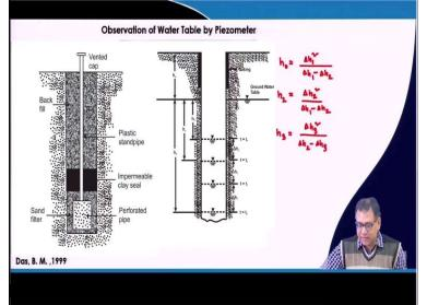
So this is the observational water table by piezometer and this is for the clayey soil where the water table or if we put the water into the borehole it will not stabilize very quickly. Suppose, this is the standpipe or piezometer inserted into the borehole and then we measure the water level at different time intervals. So, this is your borehole and we put the piezometer or the standpipe into the soil and then we measure the position of the water of this borehole at certain time intervals.
