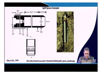
And this is the sampler tube which has 2 halves and this is the sample inside these 2 halves and these sampler tubes are pushed into the soil by hammer blow and the soil is collected from the site. So, these are the 2 couplings which are unscrewed during collection of the soil sample after taking form the site.
