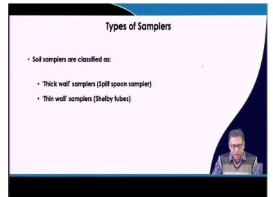
Then type of samplers so, that means, there are 2 types of sampler one is thick wall samplers, another is thin wall samplers, thick wall sampler is also known as split spoon samplers and thin wall sampler is also known as Shelby tubes.
