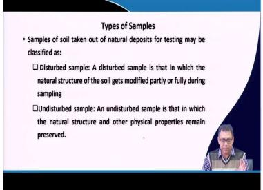
So, now, the next part so, these are the tests that I have discussed in-situ tests by which I can determine the soil sample few are directly and few are indirectly. Now, the next part and I have discussed that in several times that either we required to collect the soil sample then we have to use the sample at depth now, the question is how we have to collect the soil sample. Now, what are the different types of soil samples?
