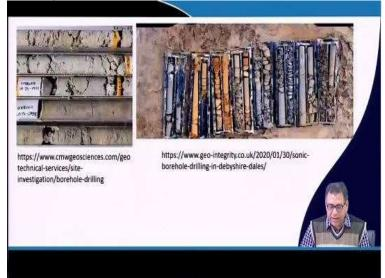
So, these are the samples and as I mentioned the inside diameter is 35 millimeter and outside is roughly 50 millimeter or 50.8 millimeter.
