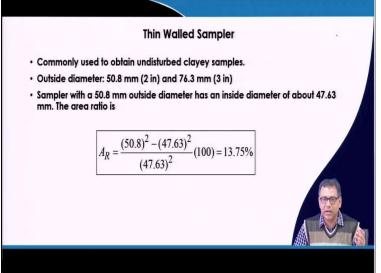
Now, for thin wall samples or the Shelby tubes, where the outside diameter is 50.8 mm and 76.2 mm. Sampler with 50.8 millimeter outside diameter and the inside diameter of the tube is 47.63 millimeter has an area ratio of 13.75%, which is close to the 10% which is the requirement. So, that means, if I use the thin wall sample or thin tube, the sample that I will get are disturbance free that means, it is a good sample or the undisturbed sample I can collect.
