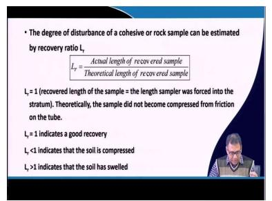
Then, by measuring the length of the soil sample also we can understand whether the sample is disturbed or undisturbed how we can identify that so, we can identify by a recovery ratio. So, this recovery ratio is equal to  $L_r$ , which is the actual length recovered sample and theoretical length recovered sample that means, if your actual length within a sampler tube is less than the length of the tube, then what will happen it indicates that the soil has been compressed.
