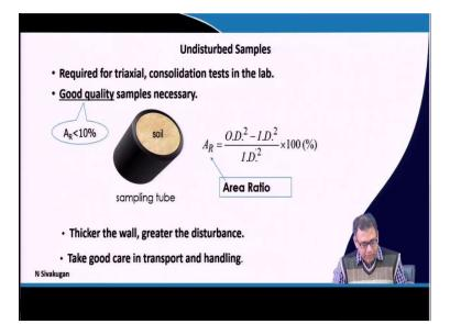
So, now the next one so, how we can collect the undisturbed soil sample what are the criteria. So, for the triaxial or consolidation test in the lab we have to collect the undisturbed samples. So, criteria that area ratio of the sample should be less than 10%. Now, what is area ratio, so, it is expected that if the thickness of the sampling tube is more than disturbed soil will also be more so, that in the sampling tube thickness will influence that disturbance.
