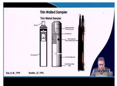
So, this is a particular sample a Shelby tube or the thin wall sample, this is the tube which is pushed into the soil to collect the soil sample.
