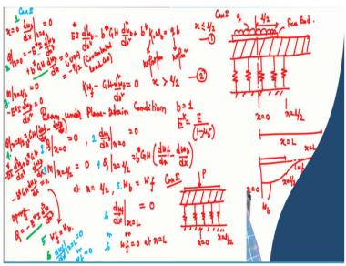
So, quickly I am giving the equations if your beam is resting on two-parameter model. So, beam on two-parameter model, your equation is  $EI \frac{d^4W}{dx^4} - b^*GH \frac{d^2W}{dx^2} + b^*k_0W = qb$ , if your q is in kN/m<sup>2</sup> and  $k_0$  is kN/m<sup>2</sup>/m. So, now here in this case, the beam is resting on two-parameter model.
