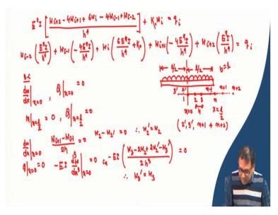
So, these equations which are expressed in central difference scheme we have to apply at all the nodes. So, this beam which has finite length is divided into number of nodes and this  $3^{rd}$  node to  $(n-2)^{th}$  node we can apply this equation, but for other four nodes we cannot apply directly this equation. So, we have to apply the boundary conditions. So, these are the four boundary conditions due to symmetry the slope is zero.
