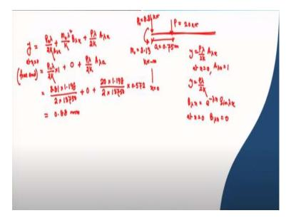
So, now finally, I will get these forces. So, P = 20 kN and this distance is a = 0.75 m. Now we have P value,  $P_0$  is 8.81, so  $P_0$  is acting here, that is  $P_0$ , which is 8.81 kN and we have  $M_0$ , and  $M_0$  is negative. So, that is why I am giving this sign. So,  $M_0$  is - 3.13 kN-m. So, as we discussed that clockwise moment to the left side is positive and anticlockwise moment to the right side is positive but here it is negative moment, so  $M_0$  is -3.13.
