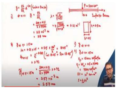
So, first problem that will discuss is an infinite beam. So, this is an infinite beam subjected to a concentrated load P = 20 kN and as I mentioned the point where the concentrated load is applied in case of infinite beam is considered at, x = 0 point. So, this is x = 0 point. So, it is in case of infinite beam. So, the width of the beam is 0.5 m that means b = 0.5 m and also, height of the beam, h = 0.5 m. So, it is a square cross section.
