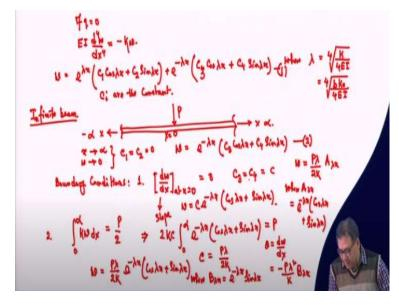
So, once I get this basic differential equation now if my q = 0 then this equation will be  $EI\frac{d^4w}{dx^4} = -kw$ . Now we can get a closed form solution of this equation, particularly this equation where external load is taken as 0, because that loading effect will be incorporated now by using the boundary condition. But right now, q is considered as 0 and I will get a closed form solution.
