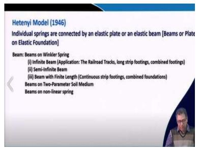
Now next model that I will discuss is Hetenyi model, where the individual springs are connected by an elastic plate or elastic beam. So, now here our beams on elastic foundation concept will start. That means here these springs are all connected with the elastic beam. For example, now these springs are connected with a beam. So, this *P* is the force which is acting.
