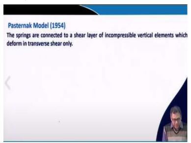
Now the next model is proposed by the Pasternak where the springs are connected with the shear layer. Because in the initial model the first model or the second model that Filolenko-Borodich model the determination of this T is very I mean confusing that which value we will consider for T. So, to represent the real soil condition, this model is more suitable or it can be applicable for this real-life problem also.
