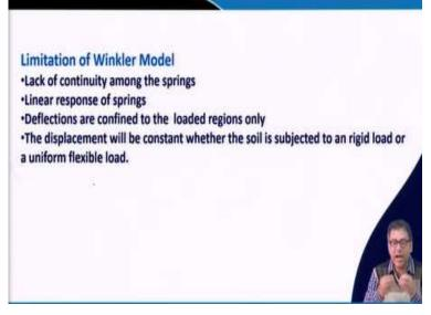
Now we are talking about the Winkler model. So, Winkler model has few limitations. What are those limitations? One limitation is there is no connectivity between the springs, but in actual foundation these springs are I mean, this soil layers are connected. That means once you apply a load on a foundation, the soil layers will deform.
