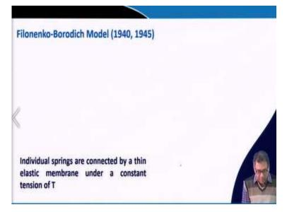
So, to remove the connectivity issue Filonenko-Borodich proposed a model where these springs are connected by a stretched membrane. Suppose these are the springs. So, these are connected by a stretched membrane, so this is equal to T. Now if you apply the load, suppose these are the springs. Now if you apply the load then what will happen then? Then not only that spring, then the outside springs will also be deformed.
