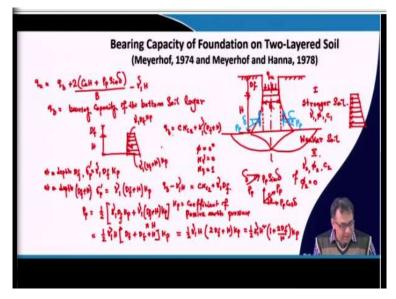
In the case 1, when the first layer is a stronger layer and the second layer is a weaker layer. And then I discussed that how the loading is acting and then because that means the bearing capacity you are getting from the contribution of the second layer that is the  $q_b$ . Then the frictional resistance that you are getting due to the movement of the soil within the first layer and that frictional resistance we are getting by using this equation.
