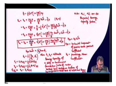
So, now if I put these values, so now I have calculated that  $P_P = \frac{1}{2}\gamma_1 H^2 \left(1 + \frac{2D_f}{H}\right) K_p$ . So, now if I put these values here, so I can now write  $q_u = q_b + \frac{2C_aH}{B} + \frac{2P_P \sin \delta}{B} - \gamma_1 H$ .
