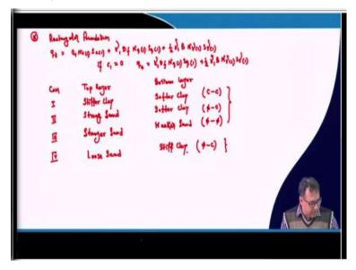
So, now for the rectangular foundation again, how we can write  $q_t$ ? That  $q_t$  again I can write as  $c_1N_{c1}$ , then shape factor we have to apply  $s_{c1}$  then  $+ \gamma_1 D_f$  then  $N_{q1}s_{q1} + \frac{1}{2}\gamma_1 BN_{\gamma 1}s_{\gamma 1}$ , 1 is for first layer, 2 is for second layer. Now, if your  $c_1 = 0$ , then  $q_t$  will be  $\gamma_1 D_f N_{q1}s_{q1} + \frac{1}{2}\gamma_1 BN_{\gamma 1}s_{\gamma 1}$ , so this is the expression.
