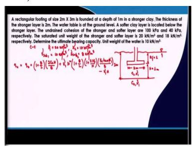
So, now let me discuss the first problem that rectangular footing of size  $2 \text{ m} \times 3 \text{ m}$  is placed at a depth of 1 m in stronger clay. So, first one is I mean it is resting on a stronger clay, the thickness of the stronger clay is 2 m, the water table is at the ground level, a softer clay layer is located below the stronger layer. The untrained cohesion of the stronger and the softer layer are 100 kPa and 40 kPa, respectively.
