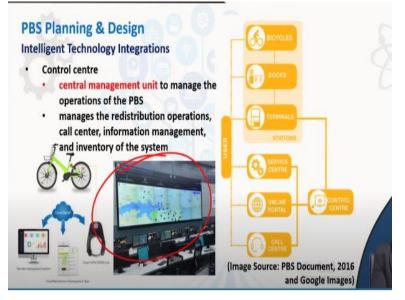
Of course, there will be a TMC, Traffic Management Center or in this case a public bicycle sharing system management center, which does all the data crunching and data analysis behind the scenes. This especially is needed because it helps in redistribution of the bicycles. It can see using the GPS tags where most of the bicycles currently are. And maybe based on the time of the day, it has to take a certain call that these bicycles have to be put in other locations.
