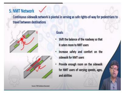
It has to have good NMT network. And we have told you in the NMT segment in the NMT module how to design good NMT network. For example, at property entrances, this is just an example of showing how property entrances should be designed. It should not be designed like this, where this is giving access only preference only to the motorized vehicle that are turning in.
