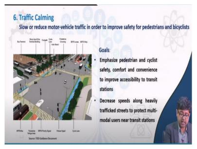
Traffic calming. We just told you in the previous classes about how to provide traffic calming devices, where to install chicanes. If you have straight roads make them a little bit windy so that traffic calms down. Essentially traffic calming is nothing but reducing the speed of motorized vehicles.
