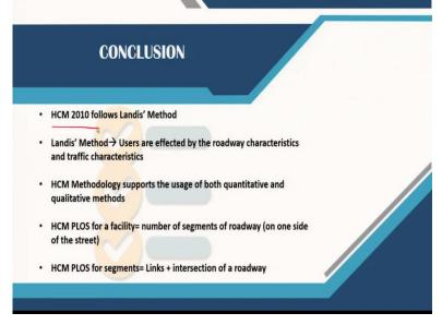
So, in this lecture, we have looked at the highway capacity manual 2010 version of how to develop a pedestrian level of service score for an intersection as well as for a link. Thank you for your attention.
