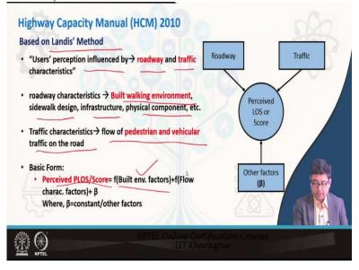
So, when we are talking about pedestrian level of service in the highway capacity manual, it is based on the Landis' method which we have already introduced to you. It says that the users'
