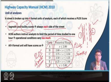
Before we do that, let us just tell you that the segment and facilities scores are always on each side of the street. Remember if there are walking facilities on both sides of the street then the segment and facility scores are different for different sites. So, that means that there may be one
