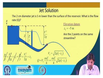
So, the jet solution, so, the question again coming back to the question, the 2 centimeter diameter jet is 5 meter lower than the surface of the reservoir. What is the flow rate Q? Again drawing the same figure, this is the elevation datum, therefore, z 2 is 5 meter below that is what it says, 5 meter lower are the 2 points on the stream streamline? Yes. So, we can write p 1/gamma + V 1 square /2g + z 1 = so, these are the 2 points just that if you are confused.
