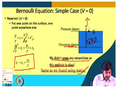
So, now, proceeding forward first simple case, very simple case, where V = 0. So, there is point 1 and there is point 2, z direction is shown as above, you know, this is pressure datum and this is elevation datum. Reservoir means V = 0. So, now, as I said this point 1 has been put on surface and we can put point 2 anywhere we have decided to put at this random point, point 2, point number 2.
