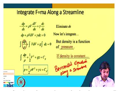
Now, we have to use force is equal to mass into acceleration along a streamline and integrate it. So, this is the equation that we have, so, what do we do? We integrate it, first eliminate ds because it is common so, we can write dp + rho V dv, because dp will come this side + gamma <math>dz = 0 and if we integrate, this will become dp. So, what we do is we divide by, you know, rho so that this gamma becomes z it will become dp / p + V dv + g integral dz = 0.
