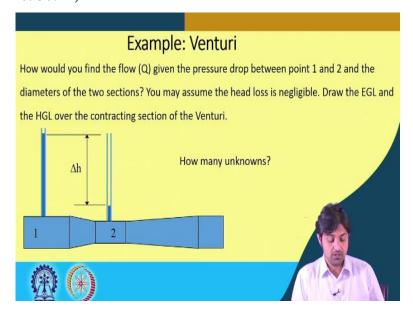
One of the examples as I said, we had not seen was venturi meter, how would you find the flow Q given the pressure drop between point 1 and 2 and the diameter of the 2 section? You may assume the head loss is negligible. Draw the EGL and the HGL over the contracting section of the venturi metre? So, this is the venturi meter, the water will rise depending upon the pressure. How many unknowns what equations are you going to use? Those are the questions.
