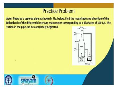
So, this is the question, water flows up a tapered pipe as shown in figure below. Find the magnitude and direction of the deflection h of the differential mercury manometer comprising to a discharge of 120 liters per second. The friction in the pipe can be completely neglected. I think we should stop the class for today now, and resume our next class by solving this practice problem. Thank you so much. See you in the next class.
