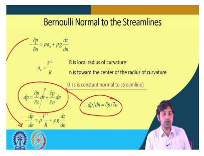
So, another concept is Bernoulli's equation normal to the stream lines. We have seen along the streamline, now the other is normal to the stream line. So, we have seen this in the previous, you know, when we are dealing with the Bernoulli's equation along the stream line. So, similarly, we can write minus the force equation we can write, - delta p / delta n + rho a n + rho n delta n + rho n and n + rho n delta n + rho n and n + rho n delta n + rho n and n + rho n delta n + rho n delta
