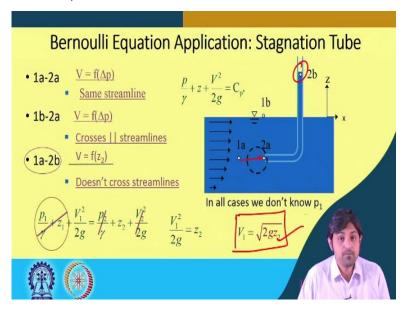
So, we assume, points 1a, 2a,1b and 2b like this, this point, this point, this point and this point. The equation, Bernoulli equation will be the same p / gamma + z + V square / 2g = constant. So, if you go from 1a to 2a, velocity will be a function of pressure, it is the same stream line; 1a is going to 1a to 2a, if you go from 1b to 2a it crosses perpendicular stream
