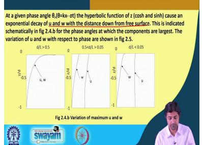
We say at any phase angle theta phase angle is  $k \times -sigma t$  the hyperbolic functions of z that is cos h and sin h cause an exponential decay of u and w with the distance down from the sea surface, this is indicated schematically in this figure. These are just the findings, you might you should not put a lot of effort and concentration and finding these values but, I mean this is pretty true right that the there is an exponential decay of u and w with the distance down from the surface.
