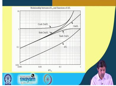
So, this is the curve which is which denotes the relationship between d by L and D by L not. So, the right hand side then this shows d by L not.
