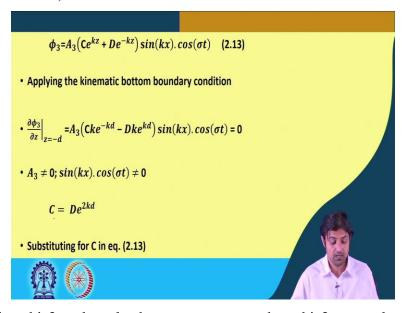
So, if we consider phi 3 and apply the same concepts that phi 3 = you know, we apply the dynamic boundary condition. This will give C equal to D into e to the power 2 k d.
