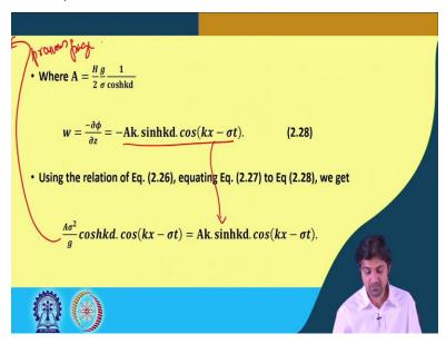
Where = be write capital A is where A is here is H by 2 into g by sigma divided one by cos h k d and w is also - del pi del z it that is - Ak sin h kd into cos k x into sigma t. And we equate this both these term A square sigma from the previous equation with this one here from the previous page because both are same.
