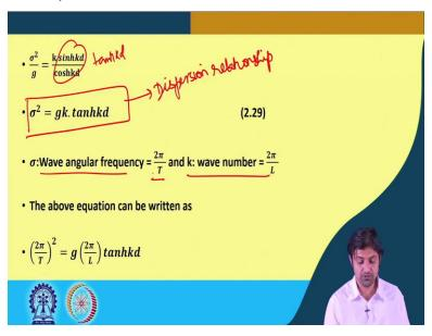
And on canceling the common terms what we get is sigma square by  $g = k \sin h kd$  divided by cos h k d and this is nothing but tan h kd. So, sigma square can be written as g k into tan h k d. Here sigma is the wave angular frequency equal to 2 pi by T and k = wave number which = 2 pi by L as we have seen before and this above equation can be written as 2 pi by t whole square = g into 2 pi by L into tan h kd. So, actually this is the famous dispersion relationship.
