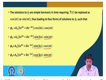
So we can write 4 different terms A1 we did not touch this, so A  $\cos k x + B \sin k x$  multiplied by either  $\sin sigma$  t or  $\cos sigma$  t. There are going to be 2 terms when we assume t as a function of  $\sin sigma$  t, and they would not mean after multiplication with this and there will be 2
