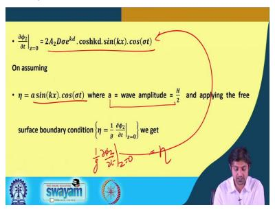
So, we have got phi 2 is 2 A2 into D e to the power k d cos h k d + z so we are left with A2 and D for now. And if we do del phi del t at Z = 0. We get 2 A2 D sigma e to the power k d cos h k d sin k x cos sigma t and on assuming if we assume that free surface elevation is A sin k x into cos sigma t. So, what we are going to do here is the wave amplitude that is H by 2 this is our assumption and by applying the free surface boundary condition that eta = one by g del phi 2 del t and Z = 0.
