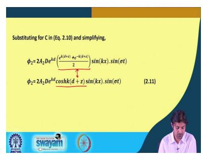
Now if we substitutes for C in equation 2.10 so instead, of CV put 2d into what the term that we have got we are going to get phi 2 = 2 A2 D into e to the power k d into sin k x sin sigma t or simply we can write this is nothing but cos h k d + z. Simple trigonometry.
