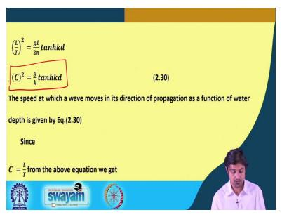
So, but is substituting since sigma and k in terms we get L by T whole square = gL by 2 pi into tan h k d or C squared =, because it can be written as C square = g by k into tan h k d. So, the speed at which a wave moves in the direction of propagation as a function of what a depth can be given by equation. Earlier we obtained the velocity potential at constant depth but now we have found out the speed of the wave as a function of water depth.
