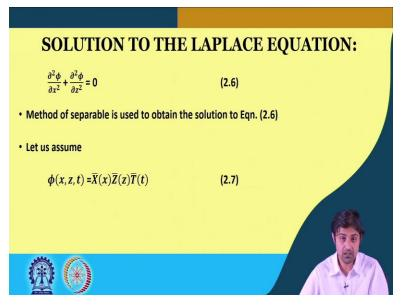
Now we have listed the boundary conditions one was w=0 at the bottom second was we specified free surface dynamic free surface boundary condition at the top. And now we start with the solution of the Laplace equation. So, Laplace equation in terms of velocity potential in 2 dimension, as we have assumed x and z is  $\frac{\partial^2 \phi}{\partial x^2} + \frac{\partial^2 \phi}{\partial y^2} = 0$ .
