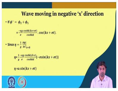
Now, if there is a wave that is moving in x direction, then we can simply write the velocity potential phi - = phi 2 + phi 1 not - phi 1 and then we will get nothing but with -  $\sin$  - ag by sigma  $\cos h k x$  sigma k x + sigma t into  $\cos h k d$ . So, what you do is you do k x + sigma t becomes k x + sigma t. So, this is a different waveform. So, in this case, since a eta is
