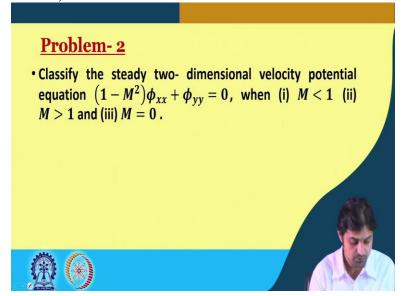
So, using this we are actually going to you know until the concepts which we have learned and now, we are going to solve this 1 question using this now so, the question is classify the steady 2 dimensional velocity potential equation, which is 1 - m squared phi xx + phi y y = 0 when m is
