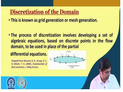
So, the second step was discretization of the domain. So, this process is known as grid generation or mesh generation. So, the process this particular process of discretization involves developing a set of algebraic equations based on discrete points in the flow domain to be used in place of partial differential equation we told that the way that it is to be done instead of partial differential equation we try to transform it into algebraic equations.
