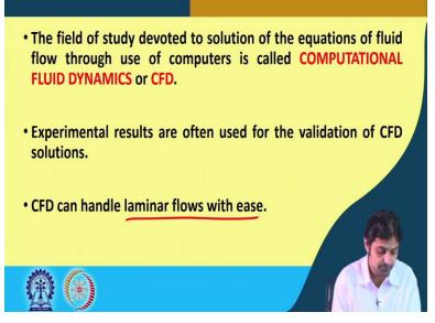
So, the field of study devoted to the solution of the equation of fluid through the use of computers is called computational fluid dynamics or CFD. So this is a very crude definition, but at your level we can say that the field of study devoted to solution of the equations of fluid flow through the use of computers is called computational fluid dynamics or CFD. So, the equations of fluid flow could be Isler equation Bernoulli's equation.
