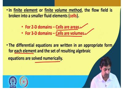
So, in finite element or finite volume method the flow field is broken into a smaller fluid element called cells. Alright. So, for 2D domain cells are areas all right, and for 3d domains, these cells are volumes. So, the differential equations are written in appropriate form for each element and this set of resulting algebraically equations are solved numerically. So the differential equations are written for each of these elements.
