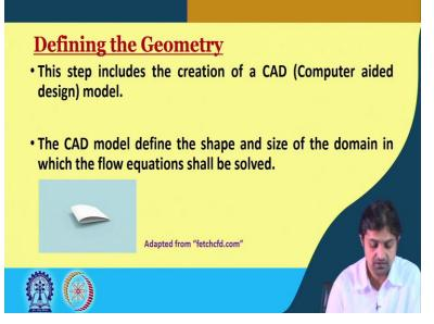
So now as we said that the first step is defining the geometry. So, this step includes the creation of a CAD model what is CAD computer aided design. So, you use some software is are there are even tools available within the computational fluid dynamics models where you can define the geometry or derive for example, suppose for example, there is a tank right and there is a pier. And you have to and this is open no I am just drawing it in 2d assume it is 3d and flow is coming through this right.
