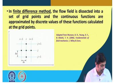
In finite difference method, the flow field is dissected into a set of grid points. And the continuous functions are approximated by discrete values of these functions calculated at grid point. So, what happens in finite difference the flow field is dissected into a set of grid points as I showed you, right so, this is 1 grid or these are grid points in x direction this is grid in y direction and the continuous functions are approximated by discrete values of these functions.
