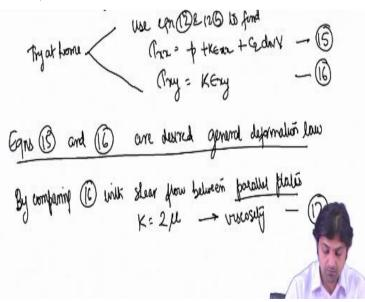
So equations 15 and 16 are desired general deformation law okay all right. So if by comparing 16 with shear flow between parallel plates we say k is 2 mu this we have done we have seen before in our topic of laminar and turbulent flows so k = and there mu is viscosity and this is equation number 17 it is just by comparison.
