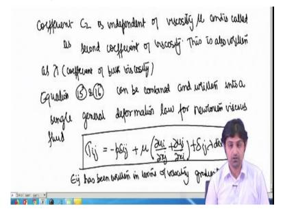
Coefficient C2 that we have mentioned before is independent of viscosity mu and is called as second coefficient of viscosity. This is also written as lambda coefficient of bulk viscosity all right. So equation 15 and 16 can be combined and written into a single general deformation law for Newtonian viscous fluid.
