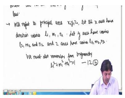
We must also remember from trigonometry 11 square + m1 square + n1 square = 1 and so on okay and this equation we called equation number 12 b all right.
