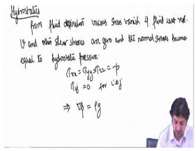
So we take a new page now and talk hydrostatics. So from fluid definition you remember the beginning definition viscous stress vanish if fluid is at rest correct. Velocity V and other shear stresses are zero and the normal stresses becomes equal to hydrostatic pressure. So  $\tau$  xx becomes =  $\tau$  yy = - pressure  $\tau$  ij = 0 for i not = j. So this implies if we put in the equation number 9 that we have obtained we become delta p = rho g all right.
