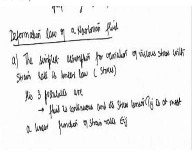
So we are going to proceed for the further derivation of the Navier–Stokes Law deformation law for a Newtonian fluid. So the idea was that we should be able to relate viscous stress to viscous strain all right. So the simplest assumption for variation of viscous stress with strain rate is linear law given by stokes. His 3 postulates are fluid is continuous and its stress tensor  $\tau$  ij is at most a linear function of strain rates  $\epsilon$  ij okay.
