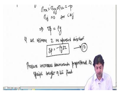
If we assume z as upward direction that means delta p will be – rho g delta z this is equation number 10. This means pressure increases downwards proportional to specific weight of the fluid and this is a very famous equation that we know from before. Now this was slight deviation, but we are going back again to the deformation for law for Newtonian fluid okay.
