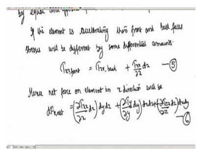
Hence, net force on element in x direction will be dFx net will be the differential right, so that is going to be now, del  $\tau$  xx x dx into dx, this is the differential stress multiplied by dy dz, same here del  $\tau$  y Y into multiplied by dy, alright into dx dz + del  $\tau$  zx by del z into dz multiplied by dx dy alright, sorry and this is we call equation number 6. So, we go to another page now.
