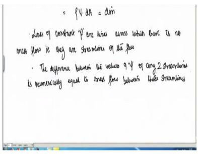
And this whole is mass flow rate, so this implies actually that lines of constant  $\psi$  are lines across which there is no mass flow that is they are streamlines of the flow. So, you are noticing in this particular module the way of approaching the streamlines and the continuity
