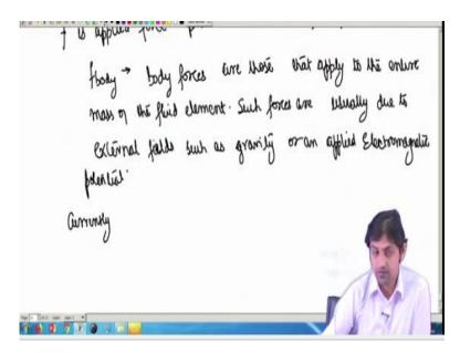
So, this f is applied force per unit volume on fluid particle, alright so, what is f body, we have to clarify that a little bit so, f body, so basically this is body force so, body forces are those that apply to the entire mass of the fluid element, okay. Such forces are usually due to external fields such as gravity or an applied electromagnetic potential, okay.
