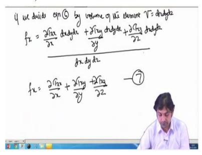
If we divide equation 6 by volume of the element, which is equal to dx, dy, dz, right we get, so differential force by unit volume we call small fx, correct is equal to; it will become del  $\tau$  xx del x, so dx dy dz + del  $\tau$  xy dx dy dz divided by dx dy dz, so dx dy dz will get cancelled from up and below both so, fx can be written as simply del  $\tau$  xx by del x + del  $\tau$  xy by del y + del  $\tau$  xz by del z and this is equation number 7, alright.
