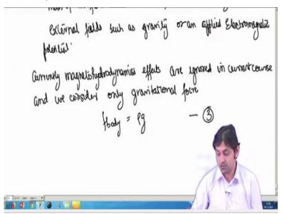
So, currently magneto hydrodynamics effects; so magneto hydrodynamics; hydrodynamics is dynamics, fluid dynamics for example, right and which is caused by the magnetic force, so these type of forces; magneto hydrodynamic effects are ignored in current course okay, current module basically and we consider only the gravitational body forces, okay. So, f body is written as rho g, alright and this we called as equation number 3, alright.
