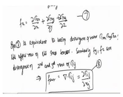
So, equation 7 is equivalent to taking divergence of vector  $\tau$  xx,  $\tau$  xy and  $\tau$  xz that means, the upper row of the stress tensor; a stress tensor is what; the tensor that we have should written here, alright. So, this is equivalent to taking the divergence of these divergence of vector I have written velocity here, a stress tensor okay, so similarly fy and fz are divergence of second and third row of  $\tau$  ij, okay.
