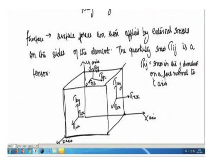
Now, the other fourth is f surface; surface force so, first the definition; surface forces are those applied by external stresses on the sides of the element. This quantity that is stress,  $\tau$  ij is a tensor, so surface forces are those that are applied by external stresses on the side of the element and this is called  $\tau$  ij, will write it in a much, alright and this  $\tau$  ij is a tensor, okay. So, let us draw a figure, I am not very good at drawing but I will try, alright.
