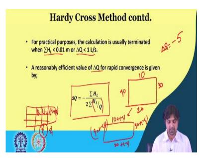
We have a led procedure in Hardy Cross Method. That will tell what delta Q is but in principle getting delta HL, sum of all the head losses exactly 0 is not possible so we terminate the calculations if we get head loss, if it is less than 0.01 meter or delta Q is less than 1 liters per second we stop the calculations there itself. So instead of 0 we go for a very, very small quantity.
