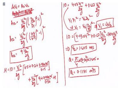
So we also know that A1 V1 = A2 V2, so A1 D1 square = A2 D2 square. So using this we can write h12 = V2 square/2g, instead of V1 sorry A1 V1 = A2 V2 sorry, so this not correct. So we can transform V1 and V2 in form of D2 and D1. So V2 square/2g, this will become D2/D1 whole square – 1 whole square. So h12 is going to be V2 square/2g and D2/D1 we all know it is 2, so 0.3/0.15 whole square – 1 whole square.
