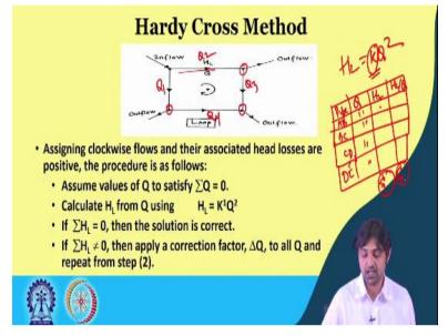
So we go back and we are going to start what we promised is like, the Hardy Cross Method. So what does the Hardy Cross Method say? So if there is a flow like this, there is an inflow and there is an outflow you see, and there is a loop that is formed. So what we do? We assign the clockwise flows and their associated head losses as positive. The clockwise flows and their associated head losses are positive.
