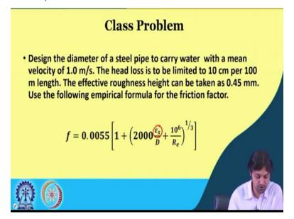
And there is one more problem. So, this is the last problem before the end of today's lecture that we are going to do. And it says is, design the diameter of a steel pipe to carry water with mean velocity of 1 meters per second. The head loss is to be limited to 10 centimeter per 100 meter
