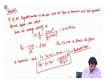
The solution 2, the first one. So, if the Reynolds number is less than 2100 the flow is laminar and the equations derived before are valid. Since, the average velocity is V = Q/A. So, Q is 2, into 10 to the power -5 and area is pi/4, into 0.020 whole square and this comes to be 0.0637 meters per second. And how do we write the Reynolds number? P VD/Mu and on putting this you will get Reynolds number, this velocity.
