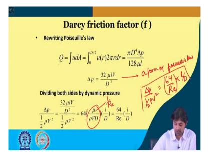
We are going to look into something here that is called Darcy's friction factor. If, we rewrite the Poiseuille's law, Poiseuille's law was pi D to the power 4 delta p/128 Mu l. Therefore, delta p could be written as, 32 Mu l V/D square, in terms of velocity. Now, if we divide both sides by this side, so this is in terms of Q and this is in terms of V. So, this is also a form of Poiseuille's law.
