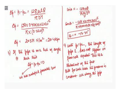
So, delta p, I will rewrite the equation, is equal to p1 - p2 = 128 Mu IQ / pi D to the power 4. So, delta p is going to be 128 Mu is 0.40, into 10 into 2 into 10 to the power - 5/pi into 10 to the power 4. So, pressure drop is going to be 20371 Newton per meter square or 20.4 kilopascal. This is the pressure drop that we found out using the Poiseuille's law. The second part says, if the pipe is on a hill of angle theta, such that, the pressure drop p1 - p2 = 0.
