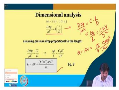
Now, the third way I said was dimensional analysis, from your dimensional analysis module. You remember that pressure is a function of V, I, D, and Mu. So, if we take delta p/l as a function of V, D, Mu or let us take, K is how much, 5, r is, so 1, 2, 3, 4, 5. So, K is 5 and r is 3. So, therefore number of dimensionless terms will be K–r, that is, 2 dimensionless term, so, pi 1 and pi 2. We get this using dimensional analysis.
