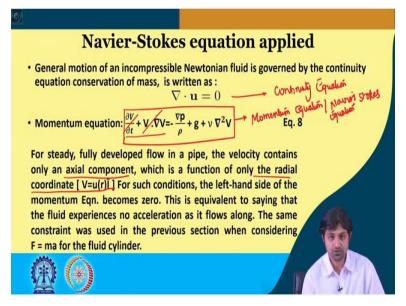
So, with this thing we are proceeding ahead for derivation of the laminar flow through pipes, using the Navier-Stokes equation. So, the general motion of an incompressible Newtonian fluid is governed by the continuity equation and the conservation of mass. This continuity equation is written as, del dot u = 0, this is continuity equation. Whereas, the momentum equation is written as, this or Navier-Stokes equation and this is equation number 8.
