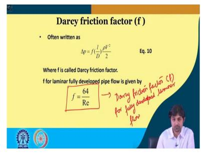
So, this is often written as, delta p = f into  $1/D \rho V$  square/2, with this equation number 10 analogy, we say that Darcy friction f for laminar fully developed pipe flow is given by 64/Re and this is Darcy friction factor f for fully developed laminar flow. And this is you must remember this.
