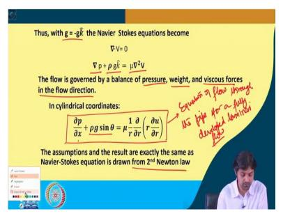
Therefore, if we write, with g as, minus g, in terms of vector, the Navier-Stokes equation, so the continuity equation will be del dot v=0 and the right hand side can be written as delta p, delta p  $+ \rho$  gk + Mu del square V. Now, the flow is governed by the balance of pressure, weight and viscous forces in flow direction. In cylindrical coordinates, we can simply write, so del p is del p del  $x + \rho$  g sin theta. Whereas, Mu in radial direction 1/r del del r into r del u/del r.
