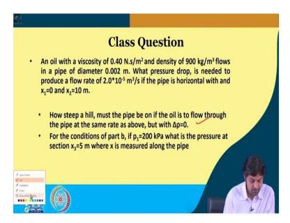
So, now, we are going to solve a question, which says that an oil with viscosity of 0.4 Newton second per meter square and density of 900 kilogram per meter cube, flows in a pipe of diameter 0.02 meter. What pressure drop, is needed to produce a flow rate of 2 into 10 to the power -5 meter cube per second if the pipe is horizontal with x1 = 0 and x2 = 10 meter? That is the first question.
