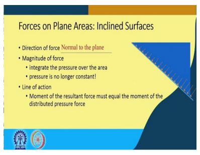
Another important thing is, we have to learn and revise again, what are the forces on the plane areas or the inclined surface. So, this has to be taken in a little bit of more detail. What will be the direction of the force? Always perpendicular, normal to the plane, right. So, the force will
