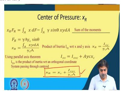
How? See, X R into F R. Where is X R? This is X R. So, X R into F R, okay. Because, yeah, is equal to integral x dF, so dF, we already know. So, it is gamma sin theta y dA, right, and this is some of the moment we know, F R is this one, gamma A yc sin theta. Therefore, x R will come out to be integral x y d A / y c A, and this is the product of inertia I xy with respect to the x and y axis.
