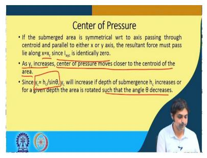
Now, the center of pressure sum. If the submerged area is symmetrical with respect to axis passing through centroid and parallel to either x or y axis the resultant force must pass a lie along
