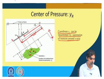
and y R is. So, let us say there is the one of the coordinates in y direction for the center of pressure centroid is here this is center of pressure right is y R, which is not equal to y c, okay. In that particular case what we are going to do is, coordinate y R can be determined by summation of moment around x axis. So, for finding y R the moment equilibrium should be done around x axis.
