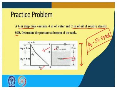
So we are going to solve some questions also, and this is quite important. So, what we say we have a 6 meter deep tank, so this is 6 meter, right? And contains 4 meters of water, so this is as it is written here very clear 4 meter and 2 meter of oil of relative density 0.88. So we have an oil the relative density is 0.88, we have to determine the pressure at the bottom of the tank. Okay? So, for your convenience we have drawn the pressure variation here on this side and this.Okay?
