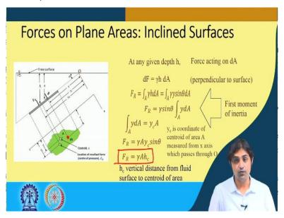
So, what I have done is, I have kept this image on the left side and how we are going to. So, for any depth h, okay. Let we say that the force acting on an area dA will be because it is at depth h, dF will be pressure into area right gamma h dA, this is the dF, this is perpendicular to the surface, that is very important. So, to find out the resultant force what should we do? We do gamma h dA integrated over the entire area, right.
