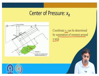
So, we also need to find out X R. What is the logical way? We will do the summation of moment around y axis now. So, for X R we need to do the moment calculation around y axis so around this axis.
