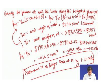
Before we go to the next concept, and that is, we have shown a manometer here in this figure. We have to calculate the pressure difference between points, M and N, this is point M and this is point N. The best way as I told you before, if you want to calculate the pressure difference or pressure at that point you have to start at one point where the pressure is known and traverse to the other point where you have to calculate the pressure.
