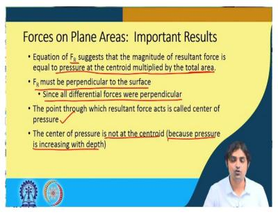
So, we proceed to the next slide, okay. So, this equation of F R suggests, that the magnitude of the resultant force is equal to the pressure at the centroid multiplied by total area. As you have seen here, see, pressure gamma A multiplied by the total area, right. F R also must be perpendicular to the surface that is very important. And the reason is since all the differential forces were perpendicular that we have counted.
