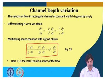
The velocity of the flow in rectangular channel of constant width b is given by, I mean, V is small q / y. If we differentiate this also with respect to x, we can obtain dV / dx is equal to  $-\frac{q}{y^2}\frac{dy}{dx}$  and if you put back V, q is V y. So, if you put this in this equation, we get this one, so it will become - V / y dy / dx. So, if we multiply the above equation with V / g, this equation by V / g, we are able to obtain this equation.
