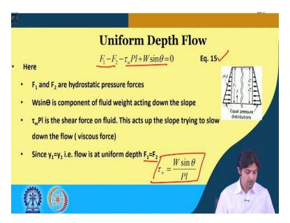
So, again rewriting the equation,  $F_1 - F_2 - \tau_w Pl + W \sin \theta = 0$  and this is equation number 15. Here,  $F_1$  and  $F_2$  are hydrostatic pressure forces, as we have already told, W sin theta is the component of fluid weight acting down the slope, tau w Pl is the sheer force on fluid, this acts up the slope trying to slow down the flow, this we have already talked about. This happens because of the viscous forces.
