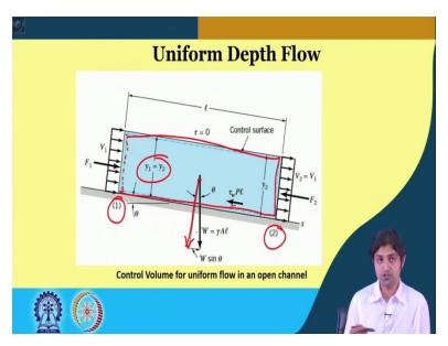
So, now, this is a cross section and we are seeing the control volume for uniform flow in an open channel. You please, we get because we are going to derive this. So, if you look at this figure very carefully, you see this is the uniform section 1 here. This is a uniform section 2, f 1 is the force, which we are going to calculate, hydrostatic force v 1 is the velocity or depth is y and y 1 and y 2, but since this is uniform depth, y 1 is equal to y 2.
