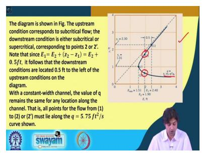
So, if we plot a diagram, we will get something like this, for this q which is 5.75 feet square per second. This is the diagram that we get, we plot we see that why critical is going to occur at 1.01 meter, the E minimum everything has been calculated if we plot this curve. So, it is, so the diagram is shown on the right hand side. The upstream conditions correspond to subcritical flow; the downstream is either subcritical or supercritical corresponding to the points 2 or 2 dash.
