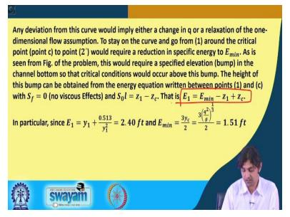
Any deviation from this curve would imply either a change in q or a relaxation of one dimensional flow assumptions. To stay on the curve and go from one, so this is the point one; the critical would require a reduction in specific energy to E minimum. As is seen from figure of the problem, this would require a specific elevation bump in the channel bottom so that the critical conditions would occur above this bump.
