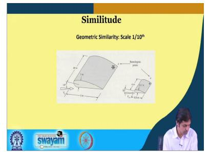
So, geometric similarity scale 1 is to 10th has been shown here. If you see, this object, this is a wink. So, you see, this length is 40 meters here and this has been brought down by 10 times therefore this length is 4 meter. I will go one by one and show you. So, this was 8 meters, this long, so, this is 0.8 meters, so, also a ratio of 10. So, this was 10 meters thick. Sorry, 1 meter thick and 10 times less is 0.1 meters thick.
