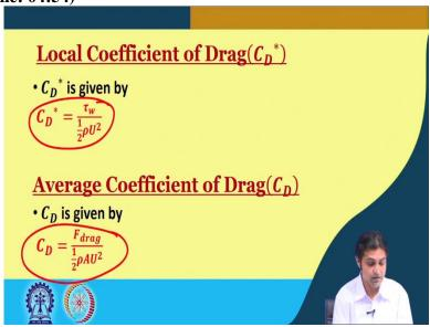
There is some, a term called local coefficient of drag C D star. So, C D star is given by, nothing, it is the ratio of tau w, the shear stress near the wall divided by  $0.5 \rho$  U<sup>2</sup>. Average coefficient of drag C D is C D is given by
