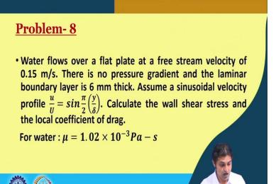
So, we start with the problem that says that the water flows over a flat plate at a free stream velocity of U 0.15 meters per second, that is, U. There is no pressure gradient and the laminar boundary layer is 6 millimeters thick. Assume sinusoidal velocity profile, like this. Calculate the wall shear stress and the local coefficient of drag. So, we have to calculate the wall shear stress and local coefficient of drag. So, how do we attack this problem?
