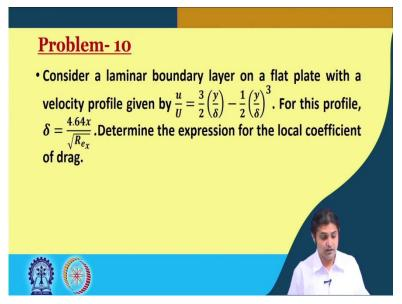
So, now, this gives us another, we will solve another problem. If we consider a laminar boundary layer on a flat plate with a velocity profile given by the cubic velocity profile, that is, what we have seen for this profile, we already know. Determine the expression for local coefficient of drag. So, how to do that?
