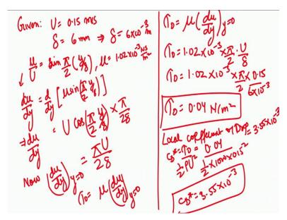
So, as always we are going to have the things that are given. So, given, U is 0.15 meters per second, delta is 6 millimeters or delta is 6 into 10 to the power - 3 meters, for example, and u / U is sin of pi / 2 into y / delta and mu here is given as 1.02 into 10 to the power - 3 Newton second per meter square. So, now, we do, du / dy, for example, that gives us d dy of u, u comes this side sin pi / 2 y / delta. So this gives us, U will come out cos pi / 2 y / delta into pi / 2 delta.
