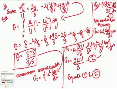
So, we have been given. So, problem number 11 is, we have been given, u / U is 2 y / delta - 2 y / delta whole cube + y / delta to the power 4. So, first thing that we calculate the momentum thickness because that is required in von Karman momentum integral equation. So, it is 0 to delta u / U into 1 - u square / U square dy. So, this profile you substitute in this equation.
