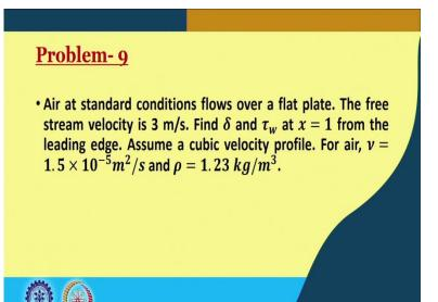
So, this was one problem. We will see another problem, which says that air at standard conditions flows over a flat plate. The free stream velocity is 3 meters per second. Find delta and tau w at x=1 meter from the leading edge. Assume a cubic velocity profile. For air, nu=1.5 into 10 to the power -5 meter square per second and  $\rho=1.23$  kilogram per meter cube.
