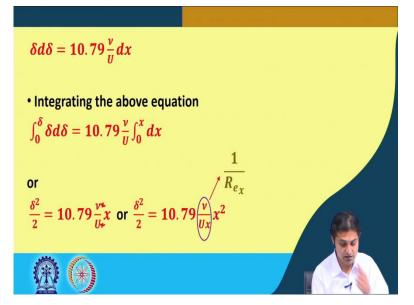
This will give us, delta d delta is equal to 10.79 v / U dx. And if we integrate this above equation, we can get the boundary layer thickness. Actually, the last problem that was their problem number 5 and 6 was exactly the same problem that we solved the way, I mean, the question was different, but the way of solving was the same as this derivation. So, we can write, delta square = 10.79 nu / U x or delta square = 10.79 nu / U x.
