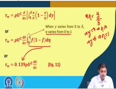
Now, if inserting the above in von Karman momentum integral equation. If we insert this, what do we get? So, tau w is written as rho U square d dx of, this is momentum thickness, theta, or in other words, you see, this is f, 1 - f d eta. Because if, eta = y / delta, so, d eta = dy
