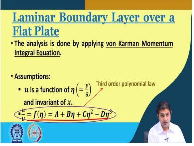
So, we will now proceed to the other topic. So, we last, when we concluded before solving the problems what we said? We said was, that the equation 1, I mean, that equation is valid both for laminar and turbulent boundary layer. So, first we study laminar boundary layer over a flat plate. So, now, this is analysis is done by applying von-Karman momentum integral equation, as it is common for both laminar and turbulent flow.
