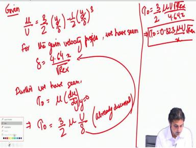
So, first write what is given to us. So, u / U = 3 / 2 y / delta - 1 / 2 y / delta to the whole cube. For the given velocity profile, we have seen that delta came out to be 4.64 x under root
