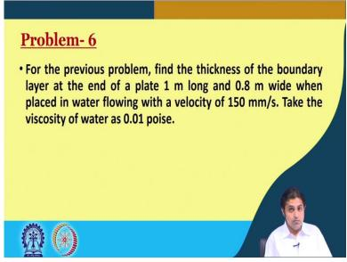
So, now, the last problem in this set is that, for the previous problem find the thickness of the boundary layer at the end of plate 1 meter long and 0.8 meter wide when placed in water flowing with a velocity of 150 millimeters per second. So, the question, theoretically we have done. Now, we need to put in some values. And it says, take the viscosity of water as 0.01 poise. So, to solve this we will go to the white screen again.
