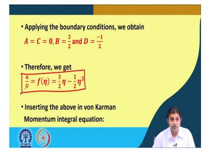
So, the first 2 conditions are going to give us A = C = 0 and substituting third and fourth. So, fourth one, the third one where we have to differentiate once, will give us this condition, you can try this at home, and the fourth condition will give us D is equal to minus 1 /2. So, those 4 boundary conditions are used to solve for these value of A B C and D. Therefore, we can simply write that, u, I mean, u / U which is a free stream velocity is given by
