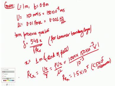
As always, we will write given. So, length is given as 1 meter, b is given as 0.8 meter, U is 150 millimeters per second or we can write 150 into 10 to the power -3 meters per second, mu is given as 0.01 poise or in SI unit, we can write, 0.001 N second per meter square. So, what we have found out from the previous question?
