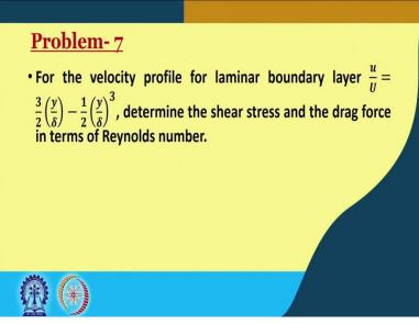
Now, we will solve 1 problem. The problem is, for the velocity profile for laminar boundary layer u / U = 3 / 2 y / delta - half y / delta to the whole cube, determine the shear stress and the drag force in terms of Reynolds number. We have done a similar problem but we will do another one now, to make it more clear.
