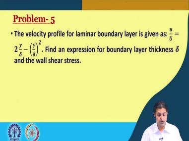
The question says that, the velocity profile for laminar boundary layer is given as u / U equal to 2 y / delta - y / delta whole square. Now, we have to find an expression for boundary layer thickness delta and the wall shear stress.
