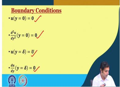
Boundary conditions. So, these were the 4 boundary conditions, if you remember. u at y = 0 is 0. Del square u / del y square at y = 0 is also 0. And u at y = delta = U and then del u / del y = at the boundary layer, the velocity gradient at the top of the boundary layer is 0. There is a free stream velocity, these two are 0. So, now, we apply this condition for also for laminar cases. What we get? I mean, this function is a third order polynomial law.
