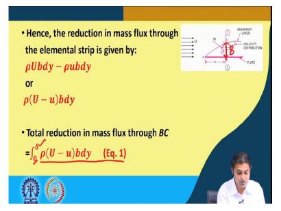
Therefore, the reduction in the mass flux through the elemental strip, compared to the, you know, uniform velocity profile will be the difference of the mass fluxes. This is due to uniform, that is, in the boundary layer, or if we take  $\rho$  outside, b and dy outside, it becomes  $\rho$  into U minus u into bdy.
