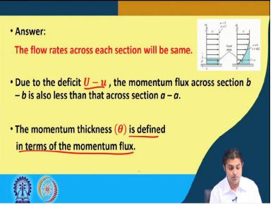
So, to answer that, we see that the flow rate across each section will be the same because the area is the same. But in this section b - b, due to the deficit U - u, the momentum flux across
