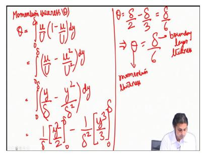
Momentum thickness theta, so, theta definition is equal to 0 to delta u / U into 1- u / U dy and this is going to be 1 to delta. This is going to be u / U - u square / U square into dy and using the velocity profile, we can write, integral 0 to delta u / U is going to be, y / delta minus y square / delta square into dy or removing the integration sign, 1 / delta would come out and this is going to be, y square / 2.
