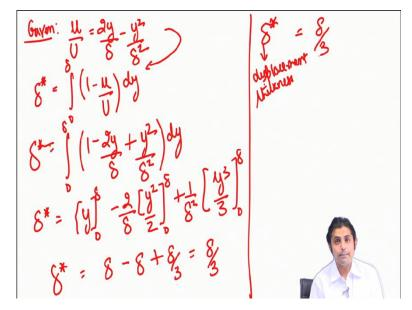
And as always, we start with the thing, that is, given. What is given to us? u / U equal to 2y / delta - y square / delta square. And according to definition of the displacement thickness, that is, delta star, definition is 0 to delta 1- u / U into dy. So, it is quite simple, we use this velocity profile here, we plug it in, and we first write, integral 0 to delta is equal to 1 - 2y / delta plus, this minus becomes plus, y square / delta square into dy. So, now there are 3 terms to integrate.
