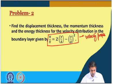
So, we proceed to the next problem. So, our next problem is, find the displacement thickness, the momentum thickness and the energy thickness for the velocity distribution in the boundary layer, that is, given by u / U equal to. So, we have another velocity profile, similar to problem number 1. So, we will solve this problem, as well. So, for doing that we are going to have white screen again.
