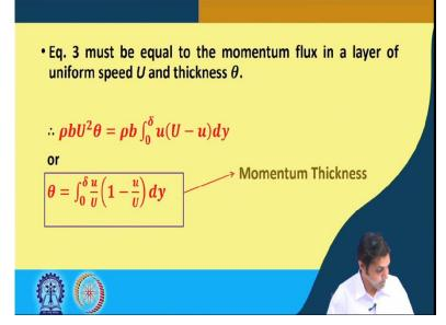
Now, the equation number 3 must be equal to the momentum flux in the layer of uniform speed U and thickness theta. That is how we derive the displacement thickness as well. So, we equate  $\rho$  b U square theta because this is the momentum flux in a layer of uniform speed U and thickness theta, or if we take this down here, as a denominator,  $\rho$  b,  $\rho$  b will get cancelled, this will become
