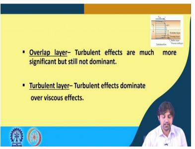
In the overlap layer, the turbulent effects are much more significant but still not dominant, in the overlap layer. In the turbulent layer, the turbulent effects dominate over these viscous effects.
