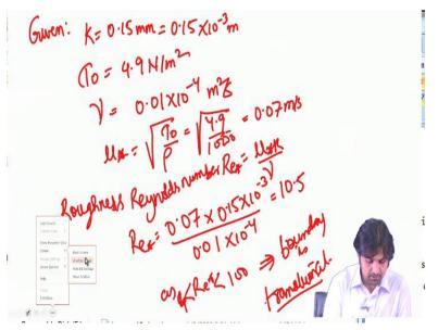
So, we have to write the things that we it has been given to us. k is given as, 0.15 millimeter, it is always a good habit to write it into SI unit into 10 to the power - 3 meter, tau not is actually
