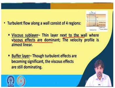
And we are going to talk about that. Turbulent flow along a wall consists of 4 regions. Viscous sublayer, this layer is thin layer next to the wall. So, this is the closest to the wall where the viscous effects are dominant and the velocity profile is all most linear. So, in viscous sub layer the viscous effects are dominant and the velocity profile is linear. In the buffer layer, though turbulent effects are becoming significant, the viscous effects are still dominating.
