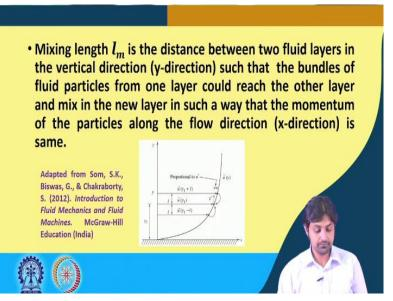
So, mixing length lm, he said it can be described in terms of mixing length l m. He said mixing length l m is the distance between 2 fluid layers in the vertical direction, in the y direction, such
