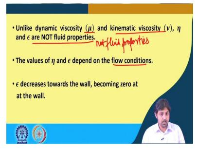
So, unlike the dynamic viscosity mu and kinematic viscosity nu, eta and epsilon are not fluid properties, they are not fluid properties. The values of eta and epsilon are dependent on the flow conditions. So, epsilon decreases towards the wall becoming 0 at the wall. So, the epsilon, that is,
