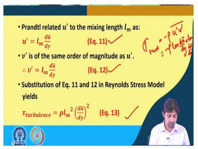
So, Prandtl related u prime to mixing length lm. He said that this u prime, as you can see in the figure here, he said proportional to u prime but I am going to write it in the next slide. He related u prime to the mixing length lm as, he said this u prime can be written as, mixing length lm multiplied by the gradient of the average velocity. So, he said u prime, this is very important to know, lm as the du bar / dy.
