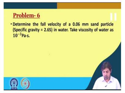
Now, we will solve a problem. The question says; determine the fall velocity of a 0.06 millimeters sand particle, its specific gravity 2.65 in water. Take viscosity of water as 10 to the power minus 3 Pascal second. This is as simple a problem as it can get. Here, you are given the diameter of the particle, we have given the gravity. Therefore, you know, the density of the particle, water properties you already know, which has actually viscosity been given already to you.
