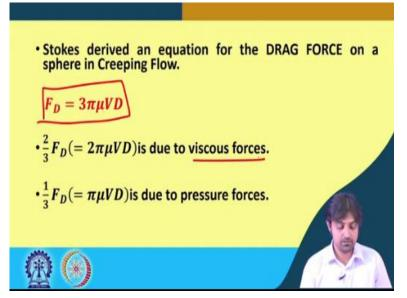
So, now Stokes derived an equation for drag force on the sphere in creeping flow. So, the derivation of the Stokes, I mean, this drag force is outside the scope. So, I am what I am going to give you directly the result. So, the drag force on the sphere is given
