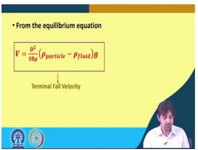
So, from the equilibrium equation we can simply rearrange these, because V is the term that we get from Drag Force equation and this is the terminal fall velocity. So, this is an important equation
