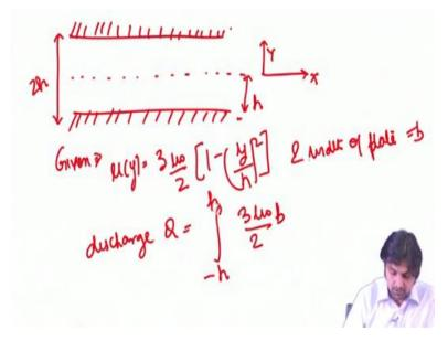
First of all it is more important to draw the plates and we draw. So, if this is the center line let us say, we are going to draw x axis in this direction, y axis is in this direction, this is h, the total thickness is 2h. So, the thickness width will be used when calculating the discharge. So, what we have been given.
