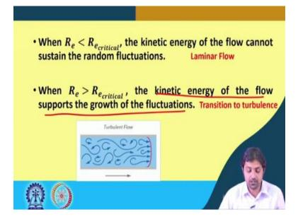
Important to know is, when the Reynolds number of the flow is less than Reynolds number, which is a critical Reynolds number, for if you remember, in the pipe flow it was 2300, the kinetic energy of the flow cannot sustain the random fluctuations and then this is called the laminar flow. When Reynolds number is more than the critical Reynolds number for example, in pipe flow it was 4000 the kinetic energy of the flow supports the growth of the fluctuation.
