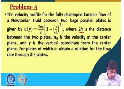
Now, we will solve one more problem, the last problem of the series of laminar flow around plates. It is a little inquisitive question. The velocity profile for the fully developed laminar flow of a Newtonian fluid between 2 large plate is given by, so, we have been given a new profile u y
