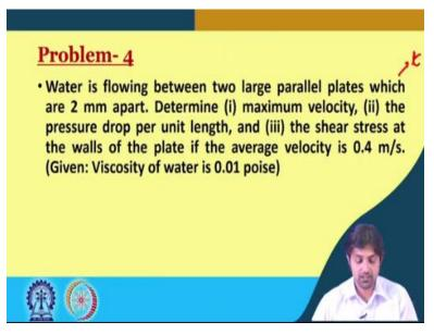
So, the question here is, water is flowing between 2 large parallel plates which are 2 millimeters apart. So, that is, means t is 2 millimeter. Determine the maximum velocity, the pressure drop per unit length, that is, dp dx and the sheer stress at the wall of the plate if the average velocity is 0.4 meters per second. And viscosity of water is given as 0.01 poise. So, to solve this, what I will go to the white screen and first write down what all things are given.
