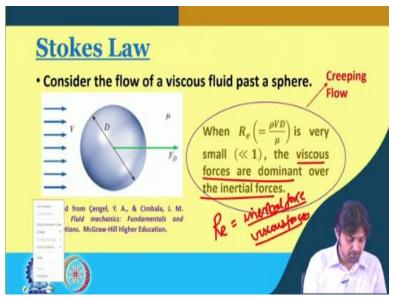
So, we now proceed to the another concept called Stokes law. So, we have to, you know, if we consider the flow of viscous flow past a sphere. So, this is the sphere and the, the flow is, there is a flow of velocity V coming to the sphere, the diameter of the sphere is D, mu is the kinematic fluid viscosity, then we will, you know, see that when the Reynolds number rho V D / mu is very small.
