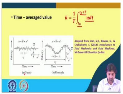
What are the time-averaged values? Time-averaged value is, if we start from beginning or time T is equal to 0 and integrate over t0 + T u dt and divide it by the whole time we get the average time-averaged value. We have done this previously when we were deriving the laminar flow we
