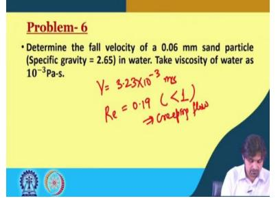
So, we have got V is equal to 3.23 into 10 to the power minus 3 meters per second and after checking the Reynolds number it came out to be 0.19 which is less than 1, therefore, creeping flow and we would have applied the terminal velocity.
