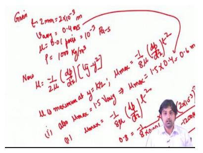
So, given thing is as I told you, t is 2 millimeters or 2 into 10 to the power minus 3 meter, the average velocity is also given 0.4 meters per second, mu is given as 0.01 poise which will be divided by 10 to obtain into 10 to the power minus 3 Pascal second, and at density of water is assumed to be 1000 kilogram per meter cube. So, we write the equation that we had derived. Now, u is written as minus 1/2 mu dp dx into t y minus y square, u is maximum at t is equal to, at y is equal to t/2.
