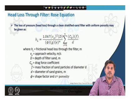
There is another equation which is Rose equation for head loss here also like we get it is a different form of equation where is based on the CD drag coefficient and as we estimated drag coefficient can be estimated based on the Reynolds number and all other things like we have known here.
