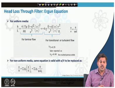
Similarly for transient state we can use the Ergun equation. So, this has a two component one is for laminar flow which is similar to the earlier one and then there is a additional component for transient on turbulent flow. So, here we have the k2 value which can be taken for crest for us what is a 0.48, a by V will be again 6 by psi d and for non-uniform media again this a by V will be replaced as this and rest of the things remains the same so similar concept is applied.
