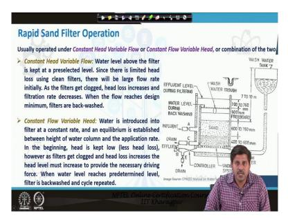
So, the rapid and operation essentially can be done in two different modes. We can operate rapid sand filters in a constant and variable flow mode or constant flow variable head mode or generally in fact these days it is more common to use a combination of these two approaches. So, filter operation is essentially like we let the influent come into the filter and then influent comes in the top.
