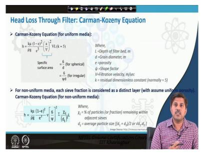
If it is falling in laminar range so we can use the Carman Kozeny or Rose equation or otherwise we can use the transient state equation. So, the Carmen Kozeny which is one of the like popular equation for estimation of the head loss so that is given as like it is in fact derived from the Darcys Westbeach equation it is a like modified version where we include for the porosity through the sand bed.
