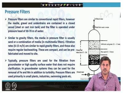
This was about the rapid sand filter, so there are pressure filters also which are very similar to the conventional rapid sand filters only difference is that the like the under drainage system the gravel system the bed everything like media bed everything will be in a closed encased container which is usually made of steel or cast iron and this will be operated under pressure. So, we can put everything in a closed container and operate the flow in the pressure.
