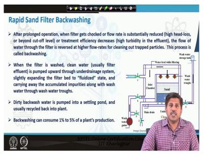
Then that means there are problems with the process so that is about regular operation during back washing again as just we discussed. So, what back washing essentially is that when we operate filter for long enough times, long enough time means, does not mean that month or year it is just 1 day, 2 day in some cases even 3 days period. So, typically 1, 2, 3 days is the operating cycle of the rapid sand filters.
