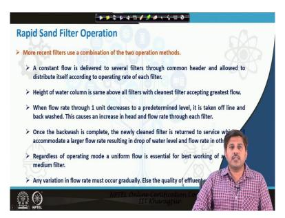
So, this is the generally like to separate mode of operation but in particularly in the recent time we use combination of these two models. So, what generally is done is a constant flow will be delivered through several filters in the common header so because we are having several filter beds it is not that we are just operating one filter bed. So, there will be several filter beds and we provide water through a common delivery head to all the filter units.
