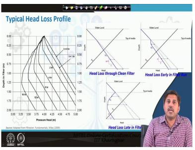
So, this is the another equation to estimate the head losses typical head losses through filtration will happen actually when we are when we are starting a new filter completely new filter so head base on the water level should be actually straight. But if we are having say this is the top of media so because of media layer we will have a reduced head. So, this is the profile of head say when the filter is started a new.
