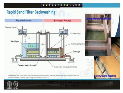
So in normal filtration we will be basically having water coming in here at the top then it will be like we allow the water flow will be this and 2 ended in a system it will be collected. Whereas in a backwash process the water will like this treated water will be pumped in this valve will actually be open and this will be pumped in and then flow takes upward and this collected water will be drained through a drainage system.
