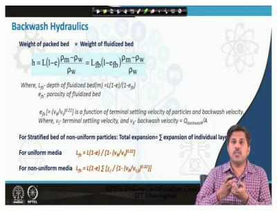
So the weight of particle is not changing so when whenever they are in the fluidized state they will have same weight. So, the weight of and that is actually going to be like weight of packed bed will be equal to the weight of fluidised bed. So, total head loss we can estimate as this or in case of fluidized it is actually this where L fb is the depth of the fluidized bed and e fb is the porosity of the fluidized bed.
