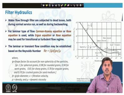
So these are like problems related to the filter operation and as we see that most of the problems are particularly like the air binding or other problems or like requirement of back washing all mostly depend on the head losses which is happening through the filter bed. So, we need to understand the filter hydraulics and how do we estimate the head losses through
