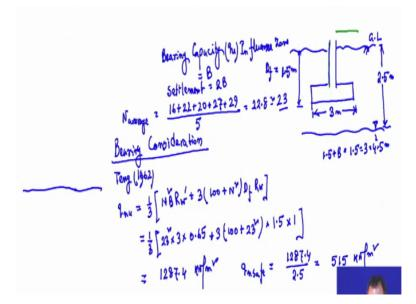
So, this is the bearing capacity expression that I am giving that for  $qnu = \frac{1}{3}(N^2BR'_w + 3(100 + N^2)D_fR_w)$ . Now here N average is 23. Now, we have to calculate the R/w and Rw. Now how we will calculate these two things? (Refer Slide Time: 23:19)
