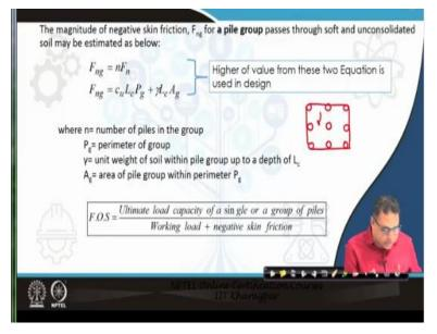
Similarly for the pile groups, the negative skin fiction can be calculated by calculating the single pile negative skin friction and then by multiplying it with the number of piles. After that, the negative skin friction should also be calculated based on the block failure which is same as the conventional pile block capacity calculation.
