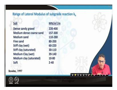
So,  $k_h$  is nothing but the subgrade modulus in the lateral direction or lateral modulus of subgrade reaction. So, the stress in the lateral direction will be equal to  $k_h \times y$ . Here, y is in the lateral direction and p is the stress acting on the pile. Here the  $k_h$  is the lateral subgrade modulus or the lateral modulus of subgrade reaction.
