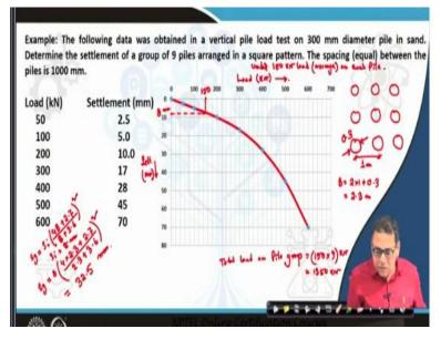
Now, let us see how to determine the settlement of the group pile using empirical expressions. The example problem shows a plate load test data for a 300 mm diameter pile in sand. The
