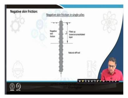
Now let us go through the concept of negative skin friction quickly. The negative skin friction is the case that occurs when the soil around a pile settles more than the pile itself. This occurs mostly when the surrounding soil is loose or is filled recently or is unconsolidated (if its) clay. If the surrounding soil is a loose sand or is recently filled, this phenomenon occurs because of the soil's own overburden pressure.
