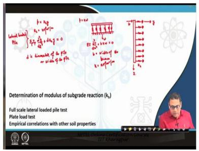
First let us see the subgrade modulus approach. Here the pile is analyzed as a beam. This is just like the shallow foundation case. So the soil, here, is represented by lateral springs but in the shallow foundation case vertical springs were used to idealize the soil. Consider that a lateral load of H is applied on the pile. For the linear analysis in the lateral direction, these spring constants are assumed to be  $k_h$ .
