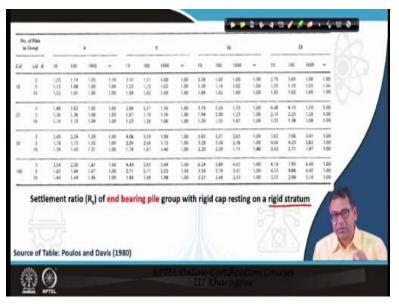
The above chart is to determine the  $R_s$  value for an end bearing pile group resting on a rigid stratum. This condition was discussed as the second case out of the three in the last class. (Refer Slide Time: 25:38)
