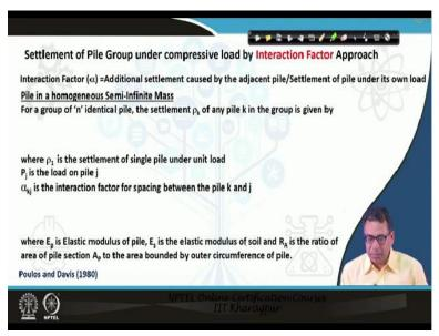
The method that is about to be discussed, with which the pile group settlement under compressive load can be determined, is called the interaction approach. In the consolidation settlement approach, the pile group is considered as a block and then is considered as an equivalent raft to determine the settlement. But there is an interaction between the piles which is not considered.
