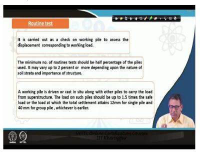
After the initial test is done, the routine test will be performed to check the working piles and to assess the displacement corresponding to working load. In this case, the test will be done on the working piles or the real piles upon which the structure will be built. So, the loading upon them should be such that it should be below failure and hence the load is restricted to 1.5 times the safe load or the load at which settlement is 12 mm for single pile and 40 mm for group piles.
