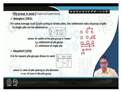
The empirical expressions are formulated from a pile load test, where if the test is done one load, the settlement of the pile can be determined for any particular load. If the total load coming onto the pile group is known and it is assumed that all the piles are taking the same amount of load or equal amount of load, the settlement of group can be determined using these expressions.
