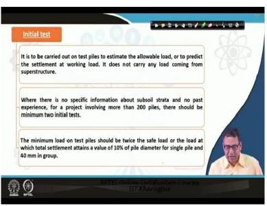
The test can be done on two types of piles and the test too consists of two parts. One is initial test that is carried on the piles to estimate the allowable load or to predict the settlement at working load. It does not carry any load coming from the superstructure. That means these are not the real
