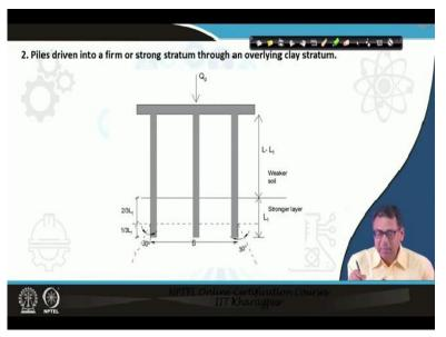
Let us see the second case in pile groups where the pile group is placed in a stronger layer at its end but passing through a weaker layer. That means that the soil profile is such that the upper layer is weaker and the lower layer is stronger. A certain part of the pile, say, of length  $L_1$  is embedded in the harder layer. Now, the stress distribution starts from a depth of  $2/3L_1$  from the level where the harder layer starts.
