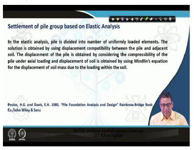
The next concept is the settlement of the pile group based on elastic analysis approach. In the elastic analysis, the pile is divided into a number of uniformly loaded elements and the solution is obtained by using displacement compatibility between pile and adjacent soil. The
