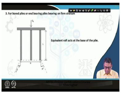
The third case is that if the pile rests on a very firm stratum of the rigid soil, then the stress distribution will be from the base of the pile. In this case, it is like the raft is placed at the base of the pile group. This is called the equivalent raft approach and it act from the base of the pile here. (**Refer Slide Time: 27:09**)
