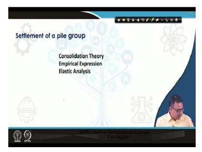
The settlement of a pile group can be determined by consolidation theory (seen in shallow foundation), empirical expressions and if the consolidation properties are not available, elastic analysis can also be used. All these three approaches to determine the pile group settlement will be discussed.
