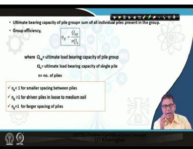
The ultimate bearing capacity of a pile group may always not be equal to the sum of individual bearing capacities of all piles in the group. The group efficiency can be calculated as the ratio of the group capacity to the individual capacity of the pile times the number of piles.
