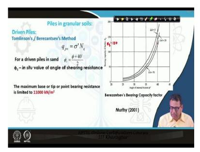
The correlation formula for the tip resistance in driven piles in granular was also given. The limiting value of the tip resistance was given as  $11,000 \text{ kN/m}^2$ .
