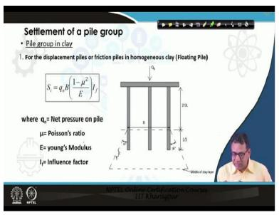
Consider a group of floating piles in a clayey soil. If a pile and its influence zone fall under a single, homogeneous soil layer, that pile can be called as a floating pile. (Floating piles do not rest on harder strata). So, if a pile group consists of floating piles, they should be first considered as a block and the stress distribution (in 1:2 ratio) from the piles to the soil is assumed to start
