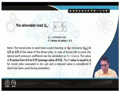
The formula for  $Q_{allowable}$  or  $Q_{safe}$  is  $Q_u$  divided by F and the factor safety is 2.5 for piles.
