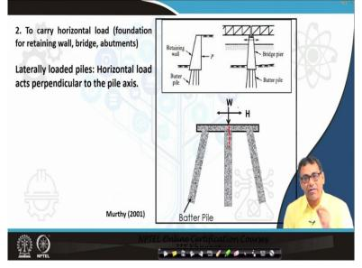
Next is about the pile subjected to horizontal or lateral load. This type of piles can be encountered with below retaining walls, bridges, apartments, or a pile in any off-shore structure where the load from a water wave acts on the pile. If the load axis is perpendicular to the pile axis, it can be called as the lateral loaded pie.
