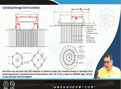
The case of a cylindrical storage tank was already discussed in the last lecture. Now, the procedure to use the boundary conditions here will be discussed. Here, the loading condition is different as the moment, concentrated load and UDL will act altogether if the tank is full. Under empty condition, again a different loading condition comes into picture.
