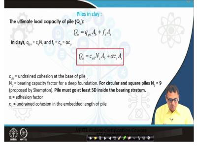
The ultimate load capacity of a pile can be given by:
