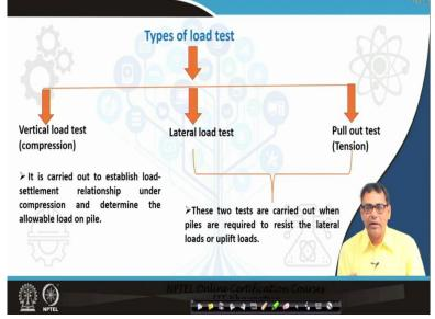
The above slide shows the different types of pile load tests through which the load carrying capacity of a pile can be determined. The pile load test is similar to the plate load test for shallow foundation but the pile load test helps to calculate the load carrying capacity of piles. There are even dynamic formulae to calculate the bearing capacity of driven piles.
