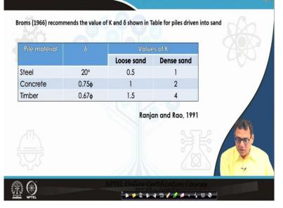
The above slide shows the table to determine the values of  $\delta$  and k for various materials and combinations.
