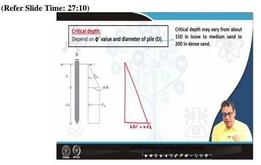
Now let us see the concept of critical depth. Usually, the lateral stress due to soil is assumed to increase linearly with depth. But in case of piles, it is recommended to restrict this value as shown in the left side figure above. So, the stress is assumed to increase up to a certain depth and then to be uniform beyond that. The depth beyond which the lateral earth pressure remains constant is termed as the critical length or critical depth ( $L_c$ ).
