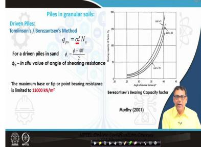
The end bearing resistance of a pile can be calculated using the correlation given above:
