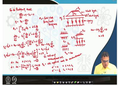
The next concept is about how to model an embankment. For the Pasternak model, the equation is:
