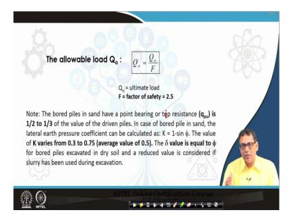
Ultimately, both the frictional resistance and end bearing resistance should be added to determine the ultimate load carrying capacity of the pile ( $Q_u$ ). This ultimate load capacity is then divided by a factor of safety (usually 2.5), to get the allowable load,  $Q_a$ .
