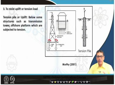
The third type of pile is the pile under uplift. Suppose there is a pile in the foundation of a tower. Due to the wind load, there is a chance that the tower will be subjected to a moment or rotation and in such case, piles in one side of the foundation will be subjected to tension. So, whenever a pile is under towers or tall buildings, they have to be checked under tension.
