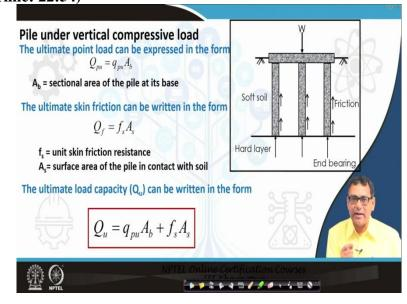
For a pile under vertical compressive load the ultimate load may come from bearing and from friction. The frictional resistance is  $f_s$  and bearing resistance is  $q_p$ . By multiplying the surrounding area of the pile, the total frictional resistance can be calculated.
