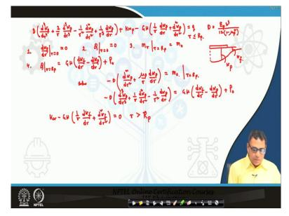
The governing differential equation for the circular tank condition will be:
