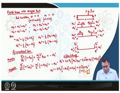
In the last class I was discussing about finite beam with hinged ends. I have derived the expressions for  $M_A'$ ,  $w_A'$ ,  $M_A''$  and  $w_A''$ . The moment  $M_A'$  and deflection  $w_A'$  are induced due to the load in symmetric case and in anti-symmetric case, the moment and deflection induced will be  $M_A''$  and  $w_A''$ .
