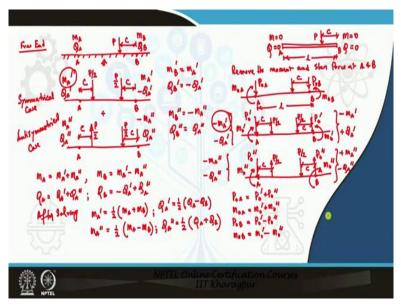
The loading condition and the expressions derived in the last class are shown in the slide above. Two loading conditions were considered which are symmetrical case and anti symmetrical case. Then the expressions for end conditioning forces,  $P_0$ ',  $P_0$ ",  $M_0$ ' and  $M_0$ " to nullify the moment and shear force at the two ends A and B were determined.
