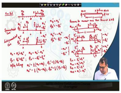
The bending moment and shear force developed at both the ends are named as per the loading condition and for the symmetric condition:
